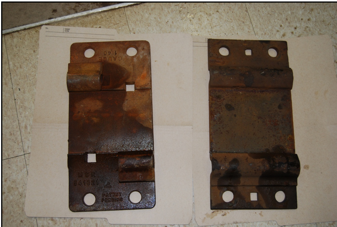
Photo 6. Cast plate (left) and rolled plate (right)
