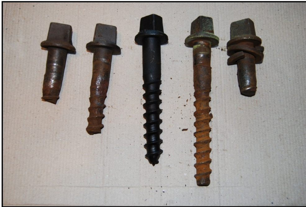
Photo 2. Broken 8.5-inch lag screws, new 7.5-inch lag screw (middle) and old 8.5-inch lag screw (2 nd from right)
