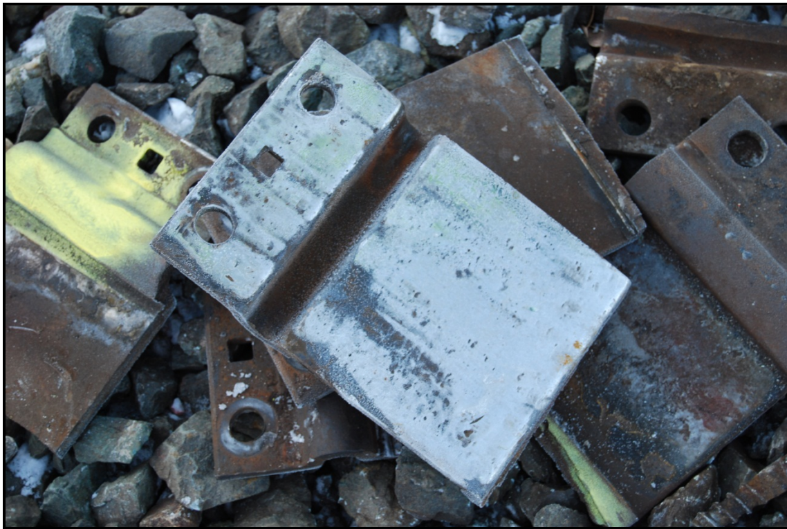
Photo 8. Shiny bottom of broken rolled plate
