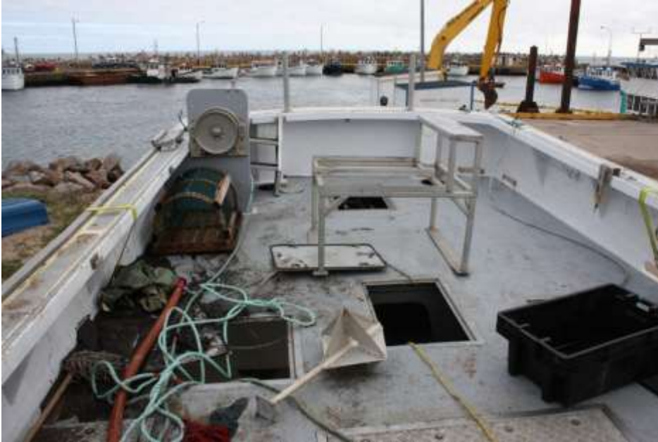
Photo 2. Working deck of Lady Jacqueline upon recovery, showing hatches with covers not in place
