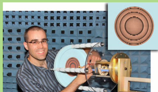
Nicolas Gagnon with a PSS Fresnel lens (insert) in a measurement jig.
