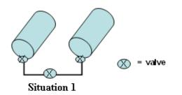
In situation 1, it is possible to isolate each tank due to the location of the valve.
