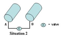
In situation 2, it is possible to isolate each tank due to the location of the valve.
