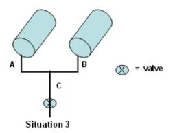
In situation 3, due to the location of the valve, it is impossible to isolate either of the tanks if you have a leak on a pipe between the valve and the tanks.
