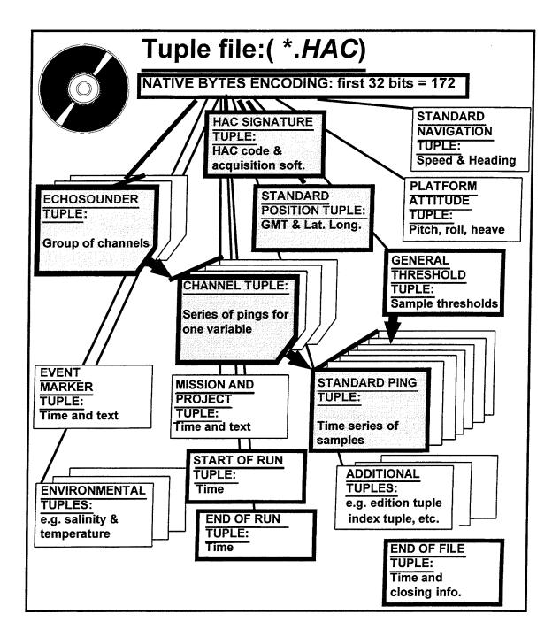
Figure 1. Organization of the information by tuples in the *HAC* standard hydroacoustic data format. The shaded tuples are required, the others are optional.
