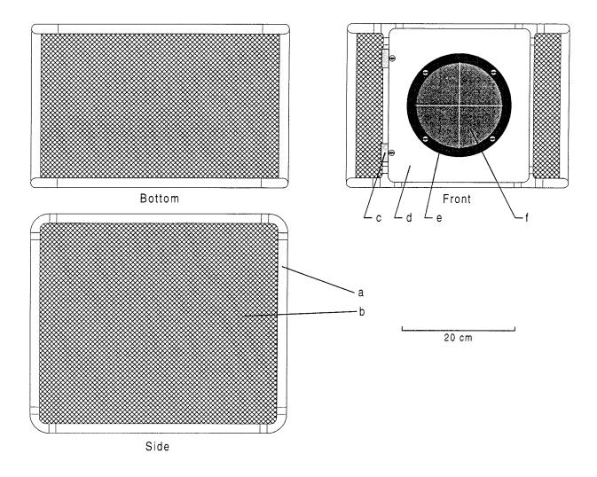
Figure 2. Details of collection cages: a) 1.3 cm dia. CPVC tubing, b) 5.0 mm nylon mesh, c) plastic hinges, d) 3.2 mm HDPE door, e) HDPE retaining ring, f) 3.2 mm rubber flap.
