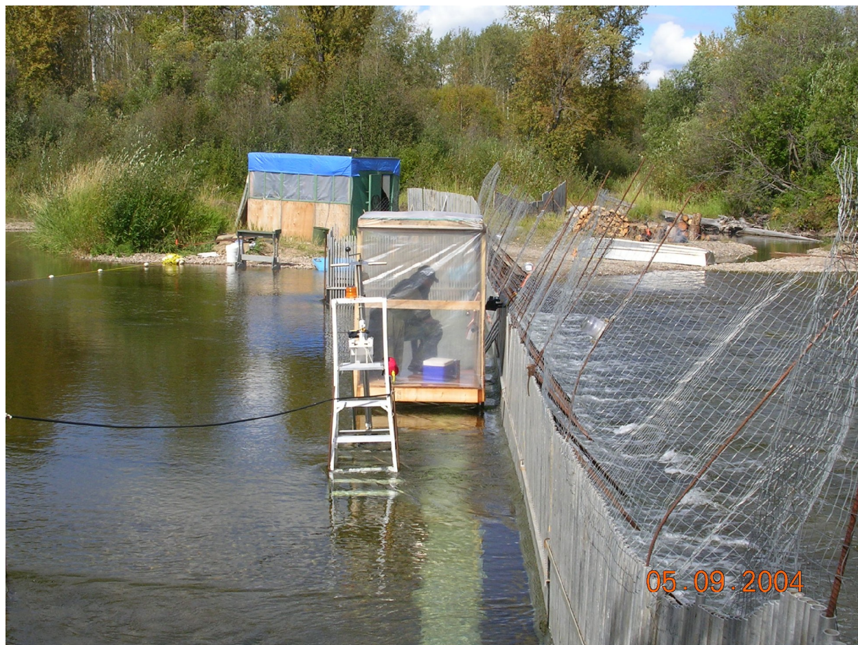
Figure 12. DIDSON equipment configuration used for count comparisons at the Stellako River Fish Enumeration Fence, 01 Sept 2004. The DIDSON equipment is about 5 m off of the right bank. Gate through which fish pass during counting is behind counting shed.
