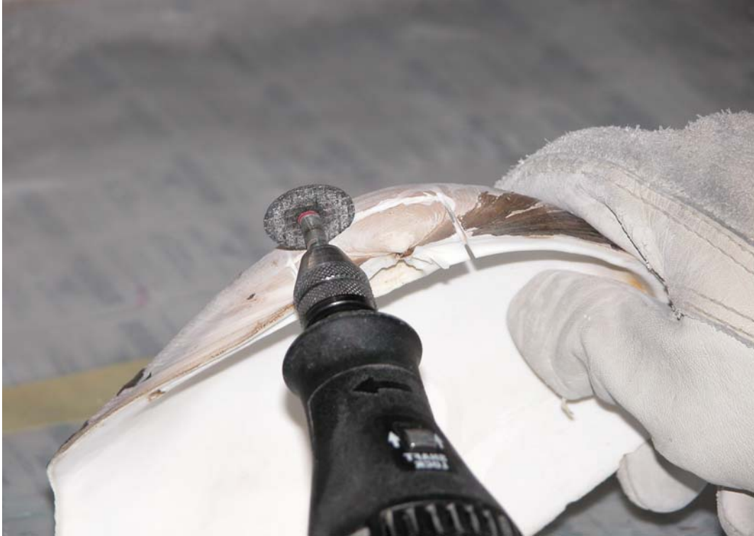
Fig. 1. Dremel® tool used to excise chondrophore from left valve.
