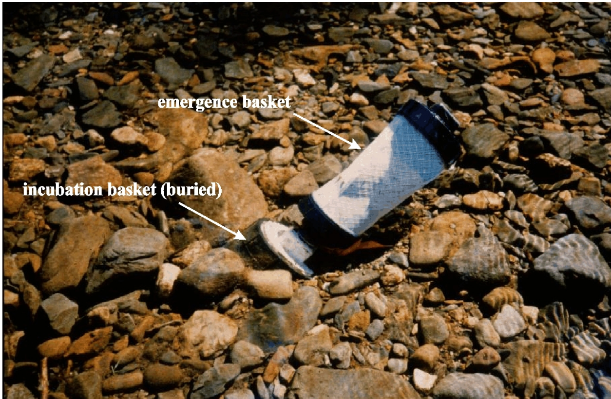
Figure 4. Photo of an egg incubation basket and emergence basket in-situ (photo taken from Flanagan 2003).
