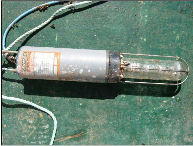
Figure 4. Aquastar aquaculture machine systems, submersible photoperiod lighting 800 W 220V-50HZ bulb type: halogen metal with Ignitor 11cm diameter 100cm length, bulb life: 12,000 h, colour yield- 90 CRI colour temperature: 6500 degrees K glass type: boro silicate. 5mm). Six of these were used in a 70 m polar circle cage holding Atlantic cod in the Bay of Fundy, near Back Bay, New Brunswick. Photo credit: O.A. Puckrin.
