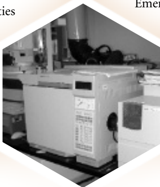
Atomic emission detector module with a gas chromatograph
