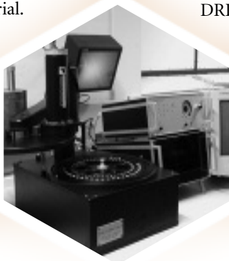
Optically stimulated luminescence (OSL) reader with single-grain attachment
