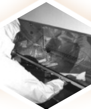
A biosafety cabinet equipped with a charcoal filter allows scientists to safely test suspicious packages
