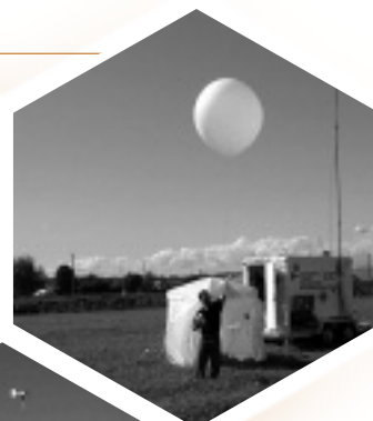
Weather balloons carrying radiosondes transmit meteorological data to Environment Canada field stations
