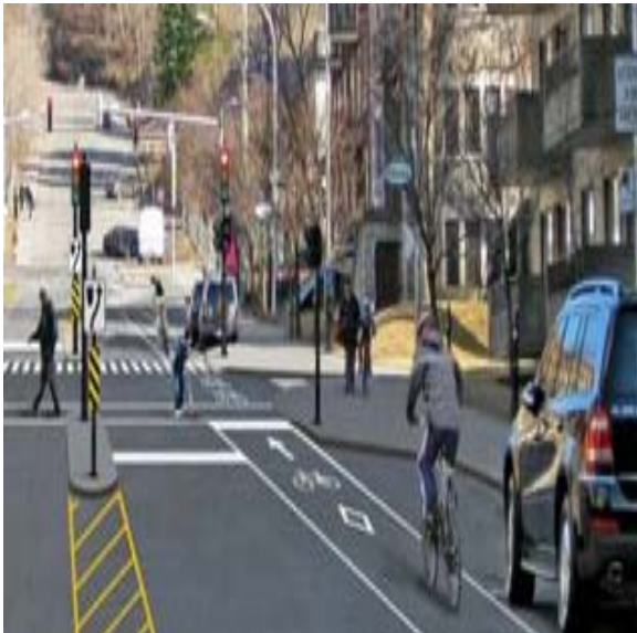
Safe intersection (simulated) The projection of sidewalk protects pedestrians and cyclists, as well as sidewalk markings and signal sequence at the traffic light.
