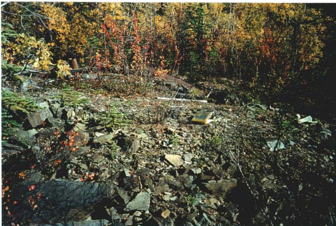
Photo 23-6: Rock dump from upper trench and adit (18m x 4m x 2m). Material comprised of approximately 80% colluvial soil and angular greenstone boulders. Photo Direction (Azimuth 120°)
