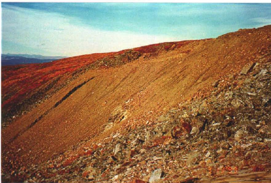
Photo 28-1: Waste rock below open cut at upper end of site. Note deep erosion path.
