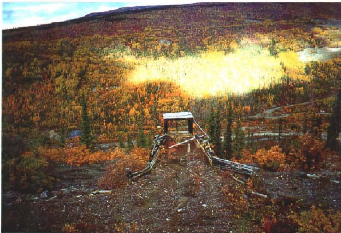
Photo 22-8: View of wooden load out from the edge of waste rock dump at Bellekeno 200 level adit (Azimuth 020°)
