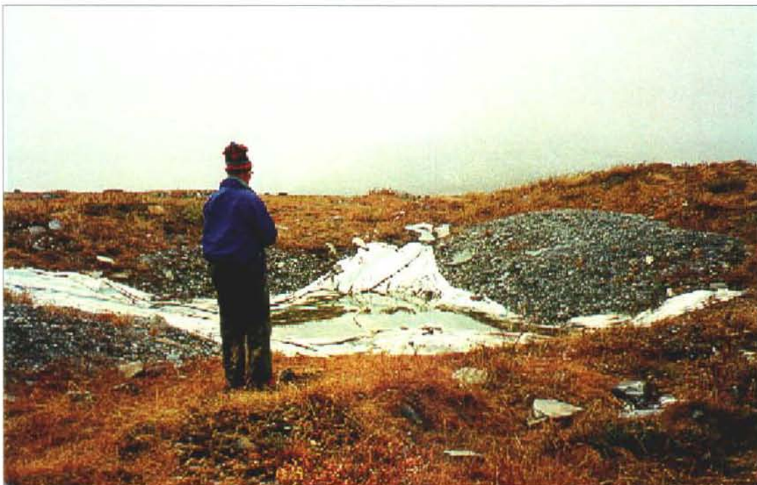
Photo 37-3 : Gold Hill No.2. Lined sump used for holding water for diamond drilling. (Azimuth 280^{\circ} )
