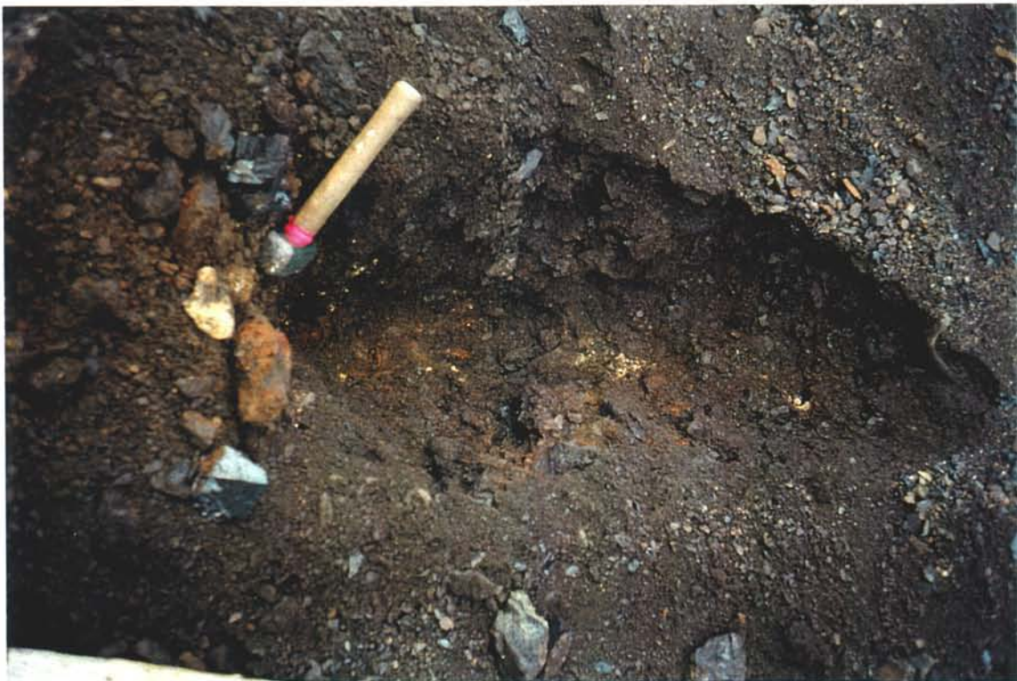
Photo 24-6: Waste rock dump WR-02 test pit (sample 24WR01-01) at Adit#2. Note strong oxidation at depth in pit and abundant siderite vein cobbles.
