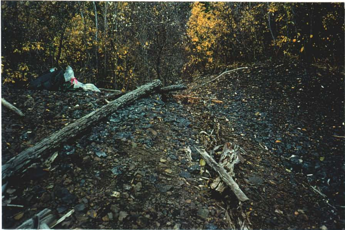
Photo 24-5: Top of waste rock dump WR-02. Note abundant manganese stained siderite vein material. (Azimuth 010°)
