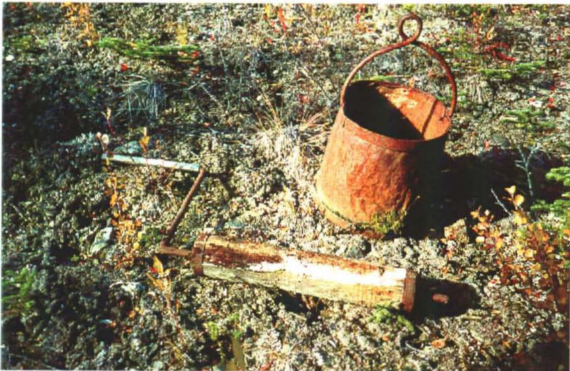
Photo 24-3: Windless and shaft bucket from backfilled shaft in area of upper trench (Shaft#1).
