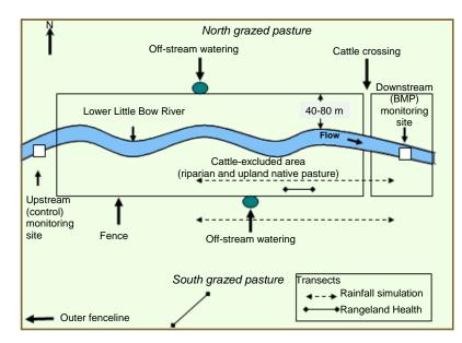
Figure 2. Schematic diagram of streambank fencing with cattle crossing
