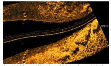
Figure 3 High frequency sidescan image of the bottom shows artificial reef material on the left (spheres) and eelgrass on the right ("clouds" with shadowed edges).
