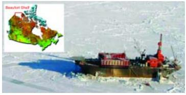
Figure 1 SDC hybrid drilling platform on location in the Beaufort Sea at the Devon Paktoa C60 well site (photo courtesy of Devon Canada)
