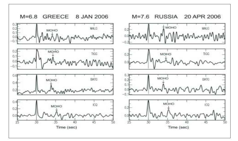
Figure 6 Comparison of radial receiver functions for several stations for recent earthquakes in Greece and Russia: locations of events are shown as yellow stars in Figure 1. The original P-wave arrival is at 30 seconds, and the Ps phase conversion from the Moho is indicated.
