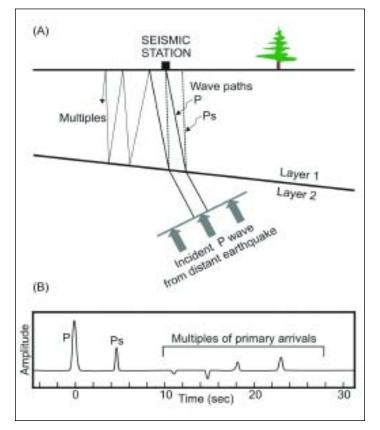
Figure 3 (A) Ray diagram illustrates the Ps conversion that is generated when a P-wave encounters a boundary. (B) The receiver function: the time difference between the direct P-wave (at T=0) and the Ps conversion provides information on S-wave velocity and depth to, and dip of, the boundary.
