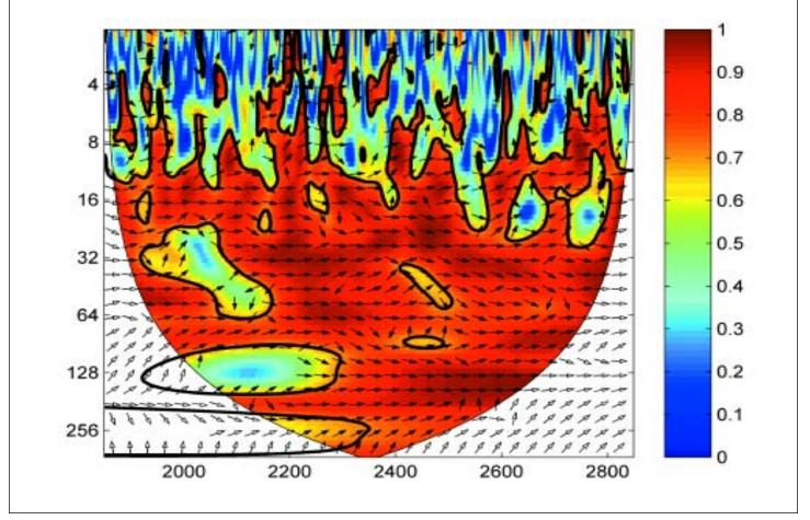
Figure 3 The colour scale (0 to 1) represents the correlation between the variables at different periods (2 to 256 years), over the thousand years. White regions represent periods with insufficient data to be statistically significant. Arrows represent the phase of the relationship: horizontal arrows left to right for variables directly correlated (in phase); right to left arrows for variables inversely correlated (out of phase).
