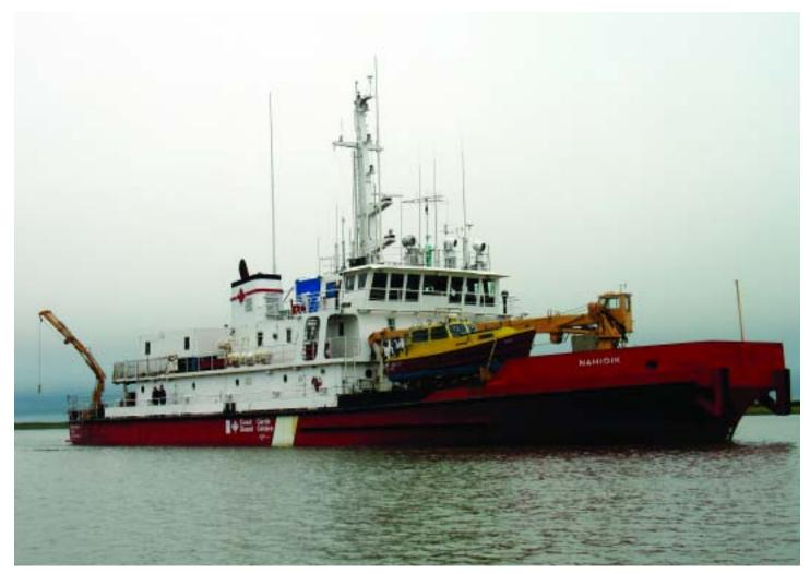
Figure 2 The CCGS Nahidik research vessel is 50 m long, has a width of 15 m and draft of 2 m. The CHS multibeam survey launch Petrel can be seen on the starboard foredeck.
