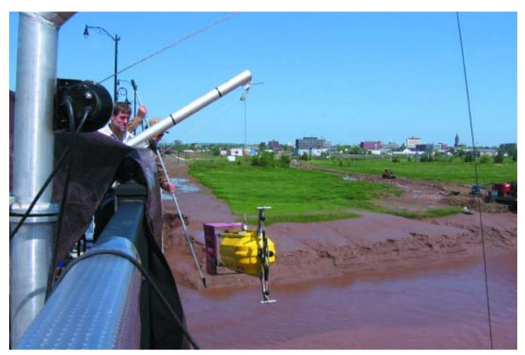
Tim Milligan and Paul Hill (behind davit) are deploying an instrument package from the Gunningsville bridge in Moncton, New Brunswick. The streamlined package contains a number of instruments designed to collect data on fluid mud in the Petitcodiac River.
