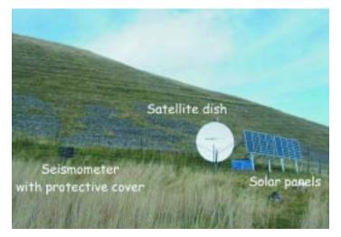
Figure 4 Station MADG on the Magdalen Islands, showing the solar panels, satellite dish, and protective cover over the seismometer
