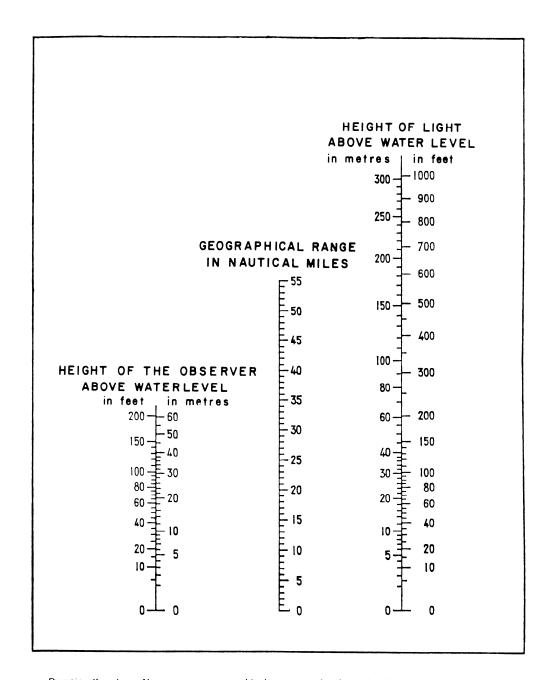
By using the above Nomogram a geographical range can be determined by placing a straightedge against the height of the respective light and the height of the observer above water level.
