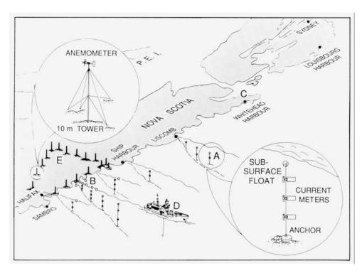
Fig. 5 The CASP oceanographers used current meters (A) to record currents and water properties every half hour for four months. Surface waves were measured by instrumented buoys (B). Sea level gauges (C) were installed along the Nova Scotia coast to record sea level fluctuations. Research vessels (D) made surveys of the temperature and salinity of the water overlying the shelf: Anemometer towers (E) recorded wind speed and direction every ten minutes.
