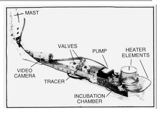
Fig. 5 The underice incubator used for measunng in situ growth rates of the underice algal layers.
