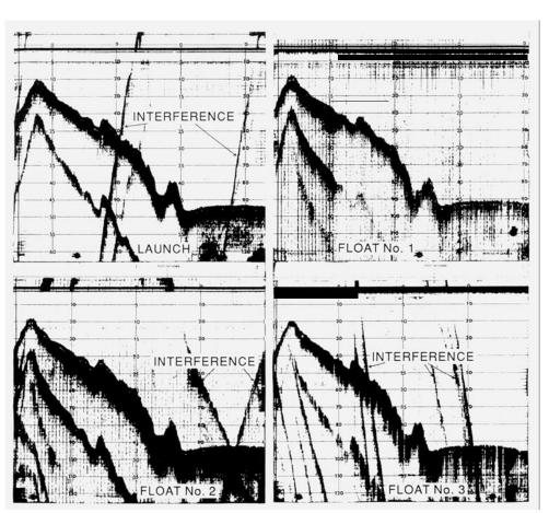
Fig. 2 Echograms from the experimental sweep system.
