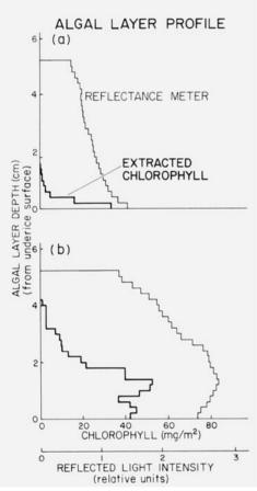
Fig. 4 Algal layer profiles determined by direct chlorophyll assay and by reflectance measurement showing (a) a narrow layer at the surface and(b) a broad layer between 1-2 cm.
