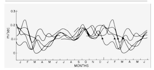
Figure 4 Smoothed records of downstream velocity measured between 1980 and 1987 at 400m depth in 1000m of water near the centre of the Labrador Current. The 18-month overlapping blocks of data accentuate the annual variation. A mark on each curve indicates where the flow drops below 0.1 m  $s^{i}$  in winter.
