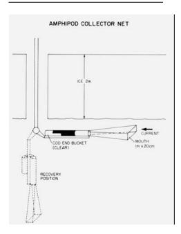
Fig. 8 An amphipod collector net used to capture amphipods at the undersurface.
