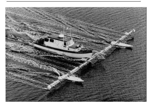
Fig. 4 The CSL Tudlik with a 30 metre boom
