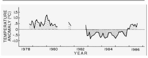
Figure 5 Monthly temperature at 200m depth west of Hamilton Bank, showing that from late 1982 through 1985 temperature was about 1°C colder than during the rest of the record
