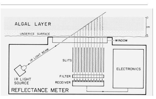
Fig. 3 The reflectance meter used to detect algal layers in the underice surface.
