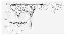
Figure 2 Temperature measured in July 1985 in a section across the continental shelf and slope at Hamilton Bank. Note the cold layer over the shelf compared to the warmer water in the deep ocean. The main part of the Labrador Current lies over the upper part of the slope, where the temperature changes rapidly from  $-1.5^{\circ}$ C to  $3.0^{\circ}$ C at 100m depth.
