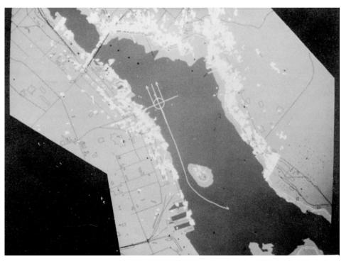
Fig. 1. Electronic Chart Testbed display of Halifax Harbour with radar. Ships symbol carries parallel index bars used to plot clear passage ahead The radar is offset 30 m east from chart because ship is positioned by GPS NAVSTAR on new satellite datum whereas chart data was on old North American datum at that time.
