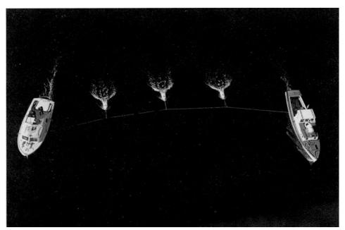
Fig. I Experimental Sweep System utilizing standard ED0 9040 echo sounders.
