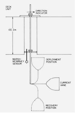
All the instruments described here and others were designed to survive the harsh Arctic environment and to be portable, allowing scientists to survey large areas of frozen waterways. Generally each of these instruments has a single unique function and measures a single parameter relating to under-ice plankton and their environment.
