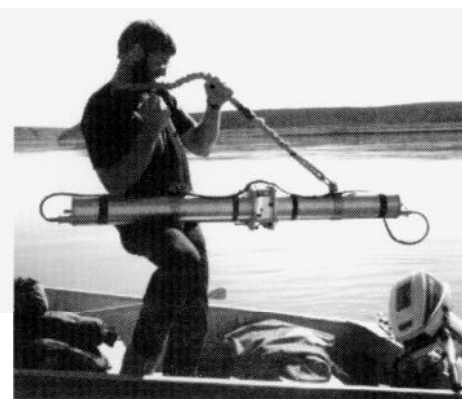
Figure 1. The deployment of the Benthos plankton camera at the confluence of the Mackenzie and Red rivers, Northwest Territories, to obtain in situ photographs of suspended particulate matter flushing through the open image area between the strobe light and the camera package.
