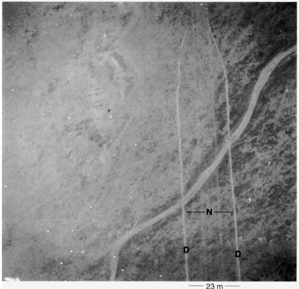
Figure 4. Track made over intertidal area off Dehaven Beach by a 18 m flounder trawl (N) and trawl doors (D). Photo from an altitude of approximately 150 m.
