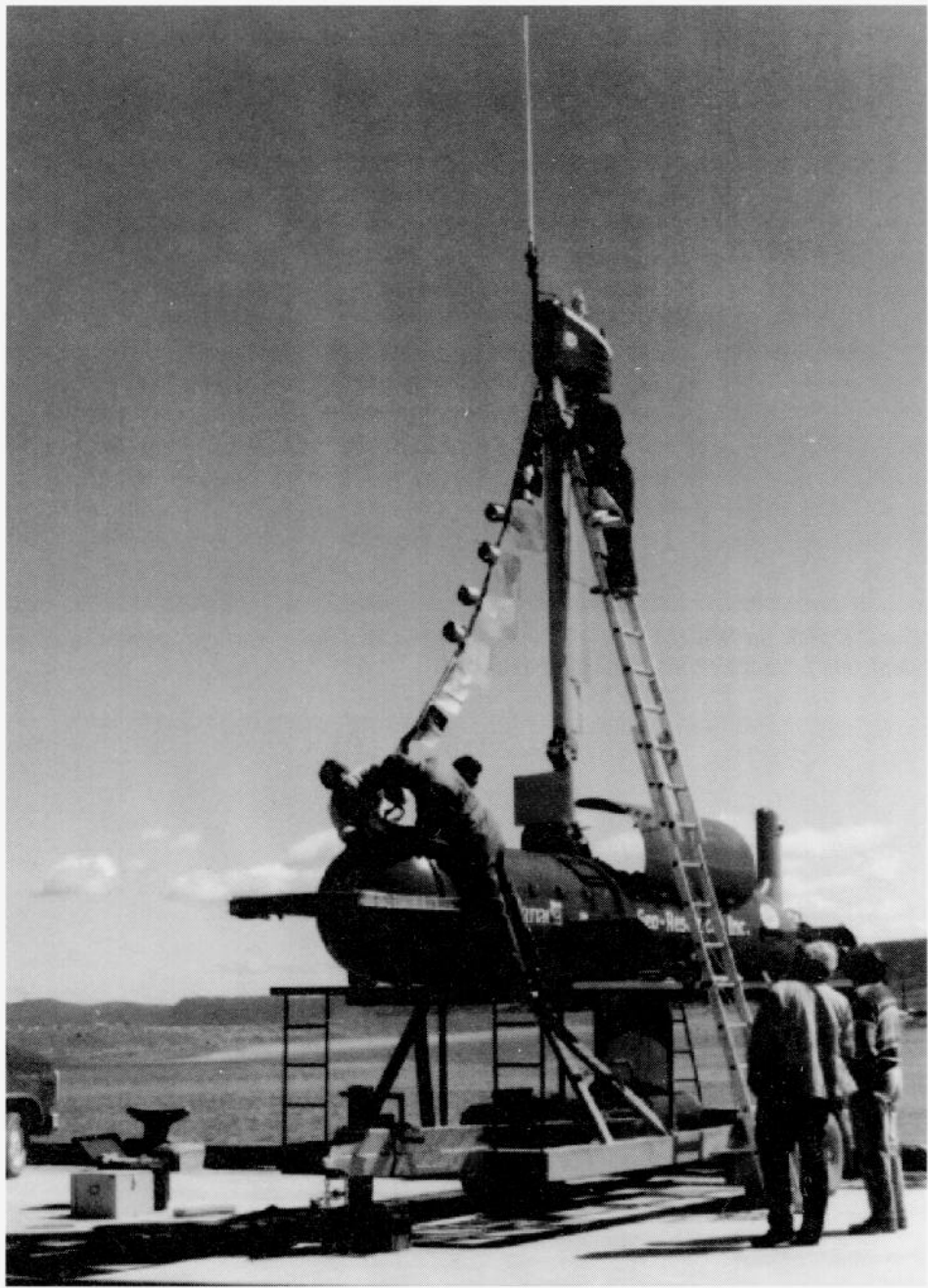
Figure 9. During a "Wave Breaking Study", DOLPHIN was equipped with side scan sonar on the keel, thermistors and void fraction sensors along the forestay, upward and downward looking sonar on the bow, and video cameras at the mast head and base. The system worked well and the data were recorded on board.
