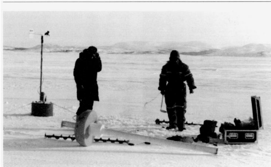
Figure 2. Ice monitoring platform being installed in ice off Labrador with an anemometer-equipped ice beacon in the background.
