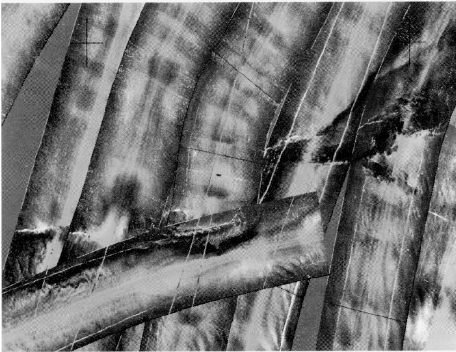
Figure 4. Mosaic of sidescan sonar data from adjacent lines. Notice how the channel can be traced throughout the mosaic.
