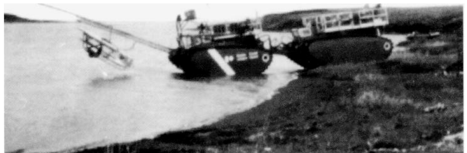
Figure 3. The Arktos-91 after modification by the Geological Survey of Canada for high-resolution geophysical surveying.
