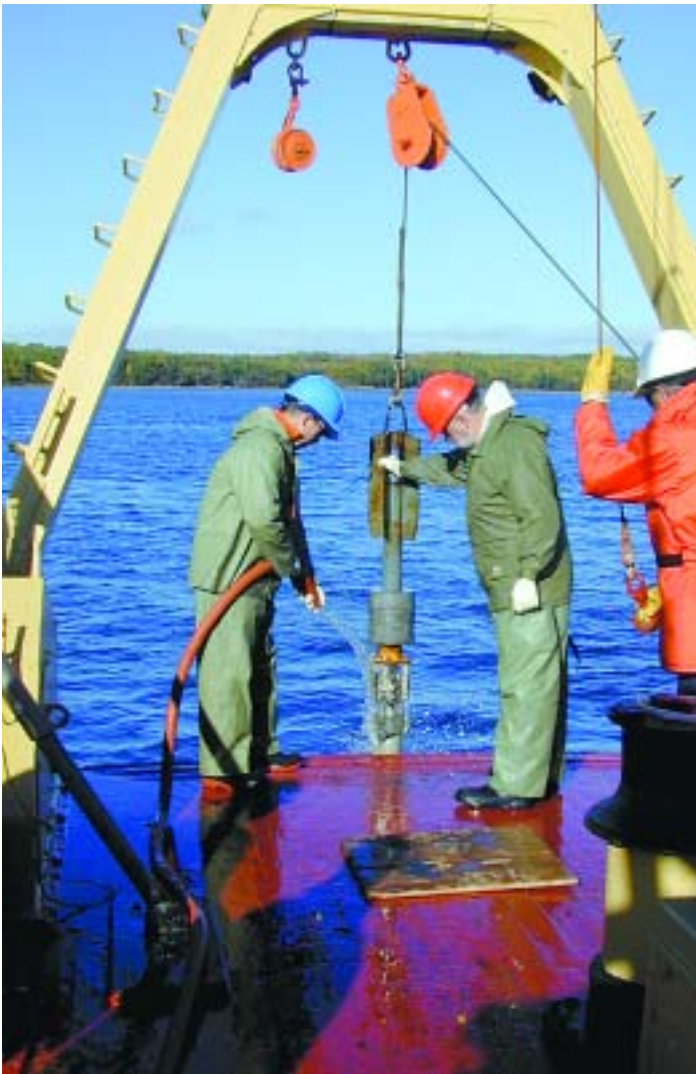
Recovery of a sediment core from Sydney Harbour by Rick Nelson, Jim Abriel, and a Navicula crew member
