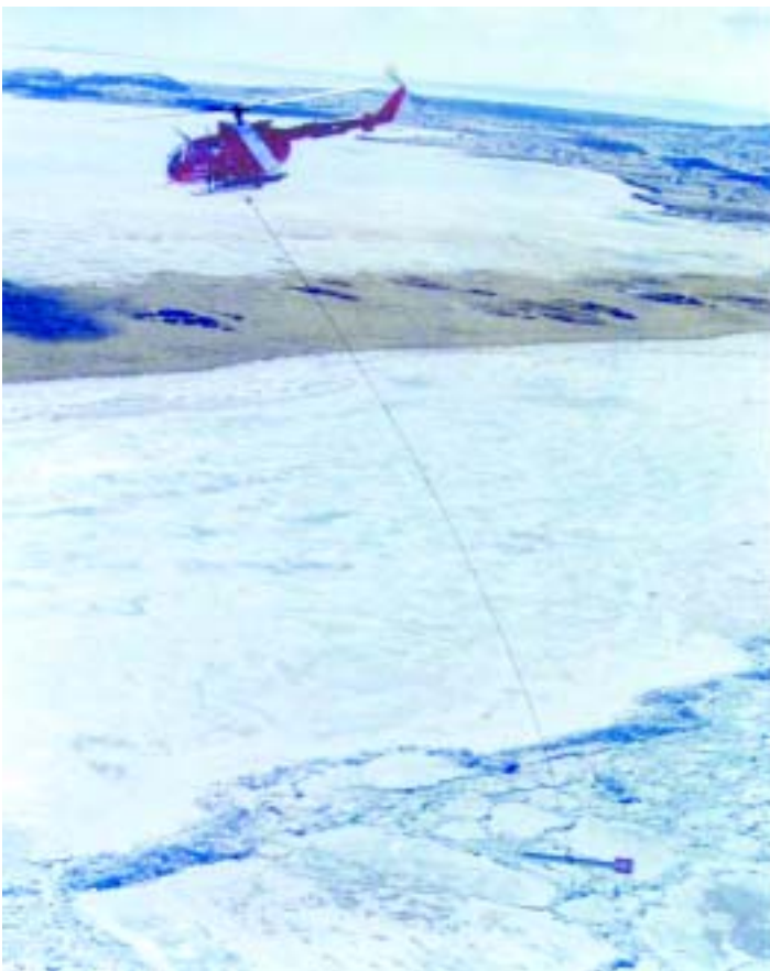
Figure 1. The Ice Probe, a towed helicopter-borne electromagnetic system for measuring sea ice thickness, is shown above sea ice in the Gulf of St. Lawrence.
