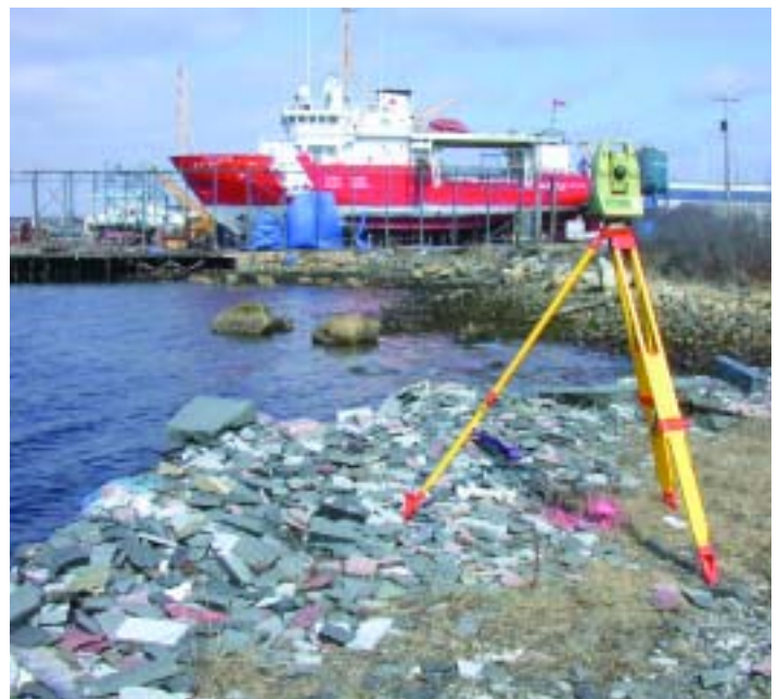
Comprehensive 3D survey of multibeam installation was conducted while Matthew was in drydock.
