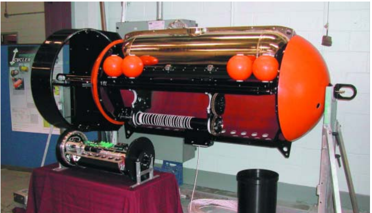
The Icycler Main Float showing the "SeaMotor" drive package in the foreground
