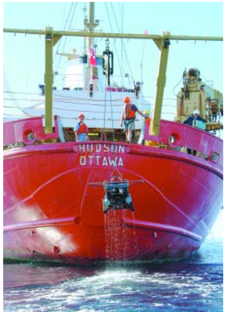
TowCam being recovered by the CCGS Hudson on the Scotian Shelf during benthic habitat studies, October 2003, Hudson Cruise 2003-059
