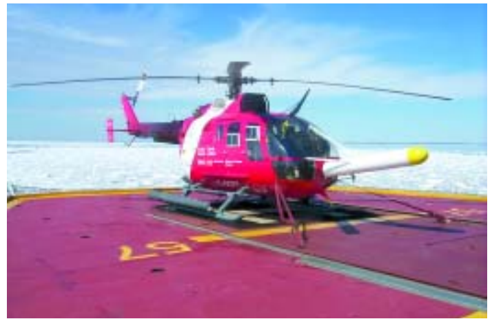
Figure 3. The Ice Pic is a fix-mounted helicopter-borne electromagnetic system for measuring sea ice thickness, shown on board icebreaker.
