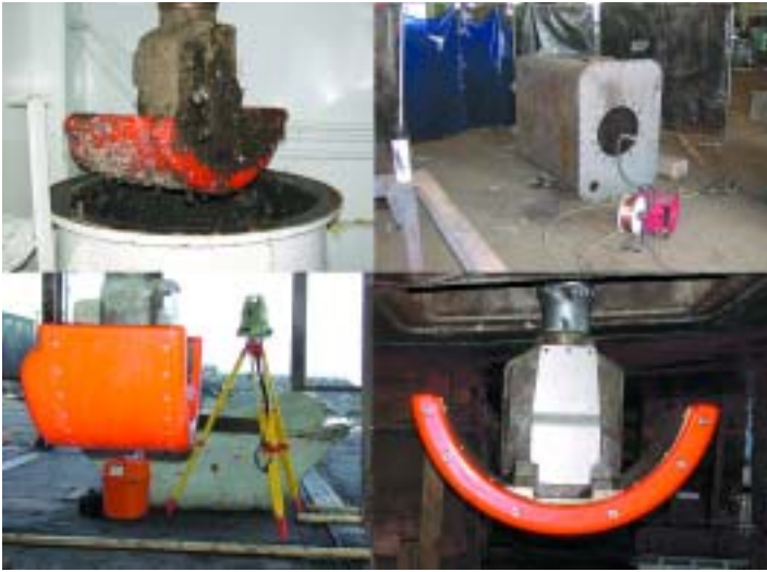
Clockwise: EM100 transducer being removed, new EM1002 trunk, two views of new EM1002 transducer installed and extended below vessel on RAM unit
