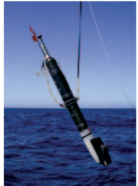
Figure 7. Prototype SOLOPC deployed in CalCOFI regional waters in September 2005 and consisting of an LOPC integrated with a SOLO drifter float
