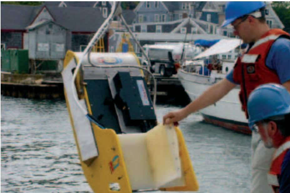
Figure 6. The LOPC mounted on a tow body preparing to survey the Hudson River
