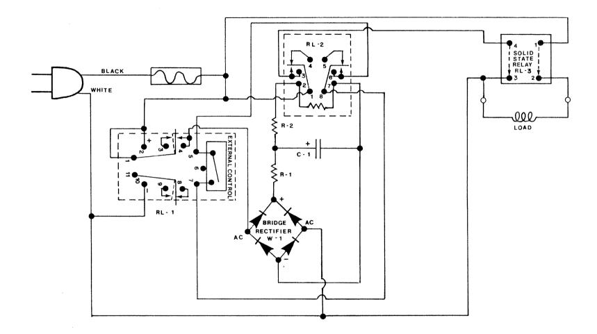
Figure 2a. Schematic diagram of the modified timing module circuit.
