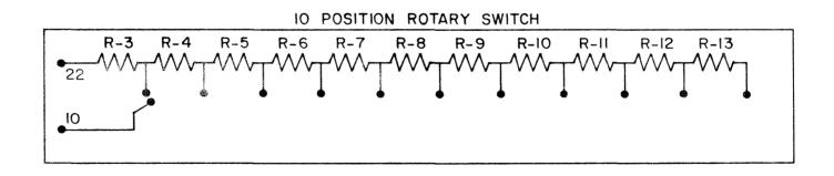
Figure 2. Schematic diagram of the timing module circuit.
