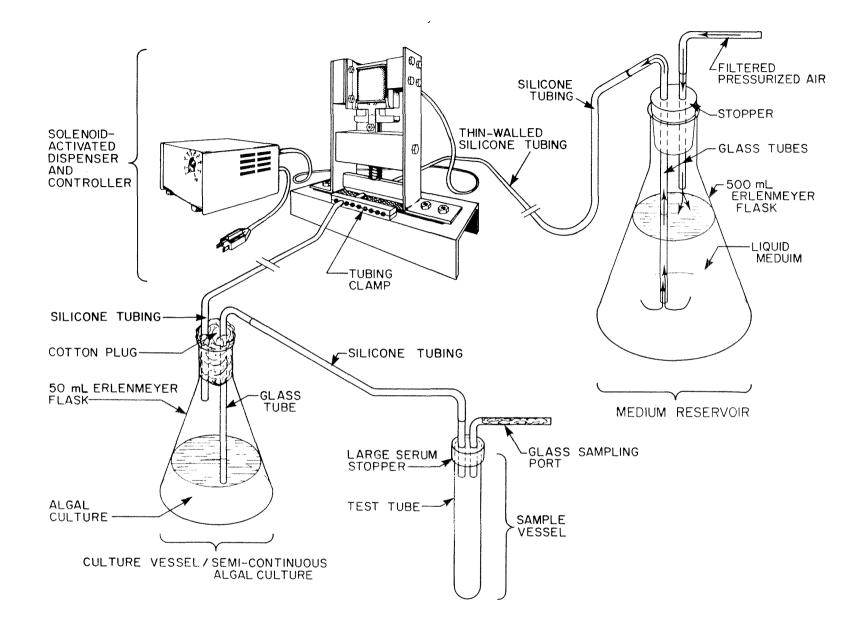
Figure 3. Diagram of the assembled components.
