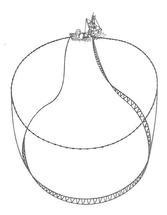
Fig. 2. Operation of a purse seine to capture sockeye salmon. A) The net is set in a circle by action of the seine vessel and its skiff. The net hangs vertically in the water with a wedge shaped opening directly under the boat.
