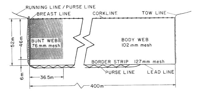
Fig. 1. Diagram of the purse seine used by the  $\underline{\mathsf{Sea}}$  Luck to capture sockeye salmon.
