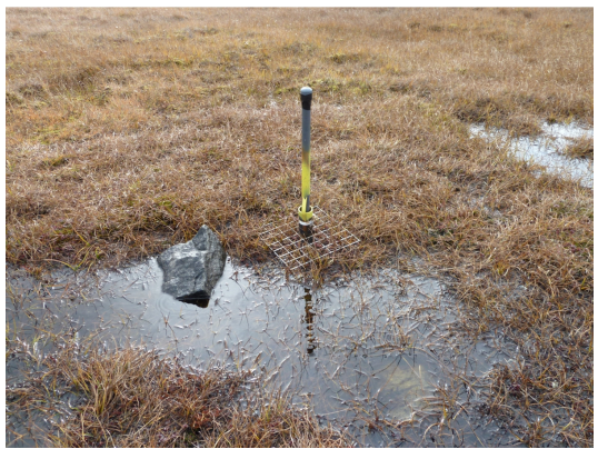
Figure 1. Thaw tube (T1) in wet and poorly drained marine sediments. See Nixon and Taylor (1994) for thaw tube description.
