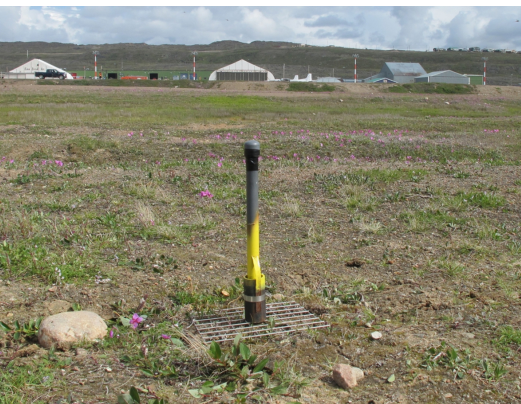
Figure 2. Thaw tube (T2) in dry and well drained glaciomarine deposit. See Nixon and Taylor (1994) for thaw tube description.
