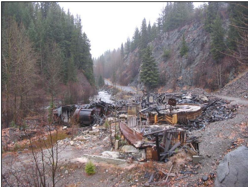
**Fig. 5.** (a) Remains of a flywheel, camshaft and cast iron mortar box from a former stamp mill (*ca.* 1900-1915) at the Lorne Mine property (now part of the Bralorne Mine). (b) Ruins of the former cyanide treatment plant (operated from 1928-1962) at the Pioneer Mine on Cadwallader Creek.
