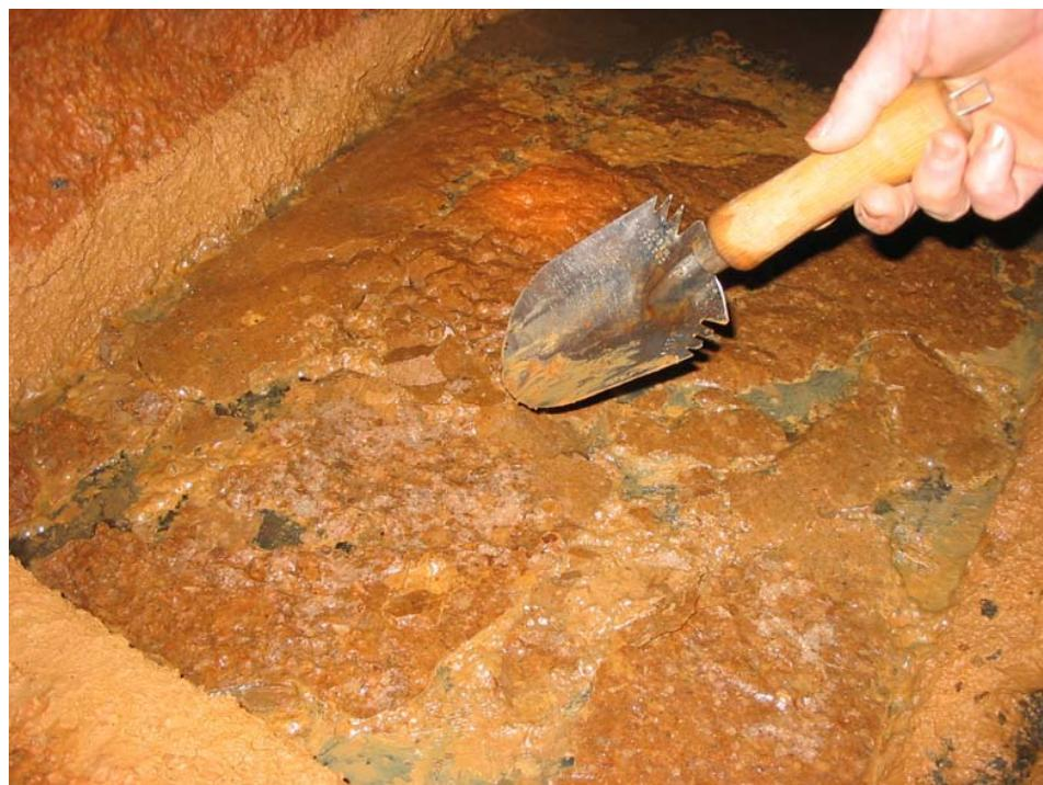
**Thin, Fe-rich crust floating on mine drainage adjacent to tracks**
