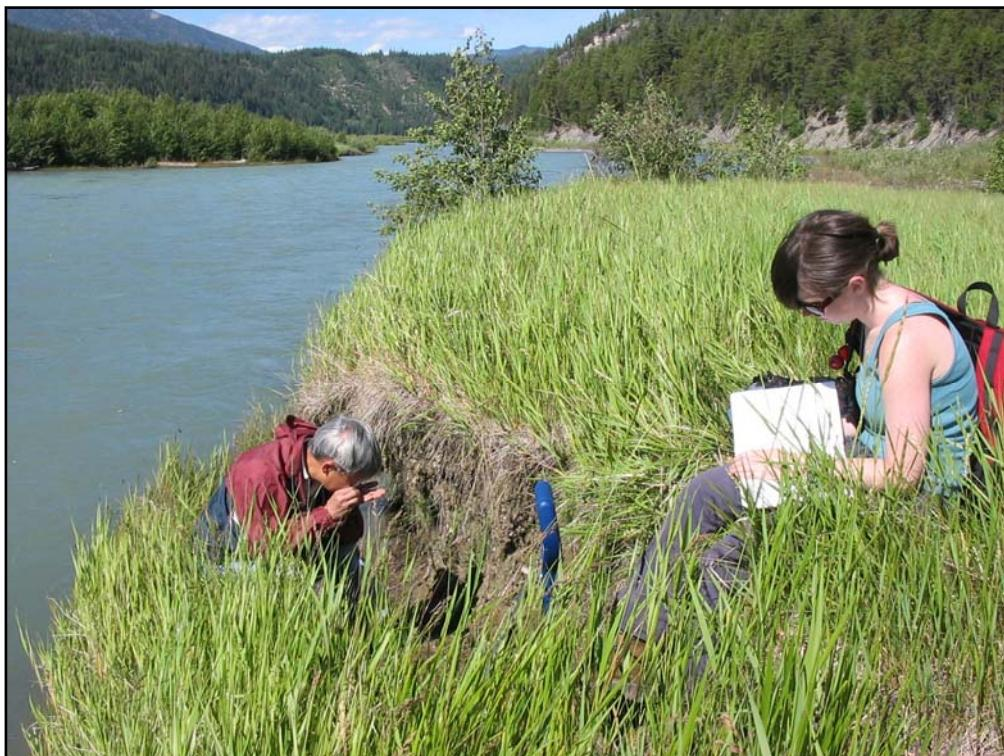
**Fig. 20.** (a) Floodplain deposits consisting of overgrown coarse, sandy sediments and tailings with abundant Fe-oxides along Cadwallader Creek, just downstream of the Pioneer Extension Mine (Sites SS27, SS28; Fig. 14, Appendix A). (b) Sediments on grassy floodplain of Bridge River, approximately  $\frac{3}{4}$  km northeast of Gold Bridge (Sites SS16-19; Fig. 13, Appendix A).
