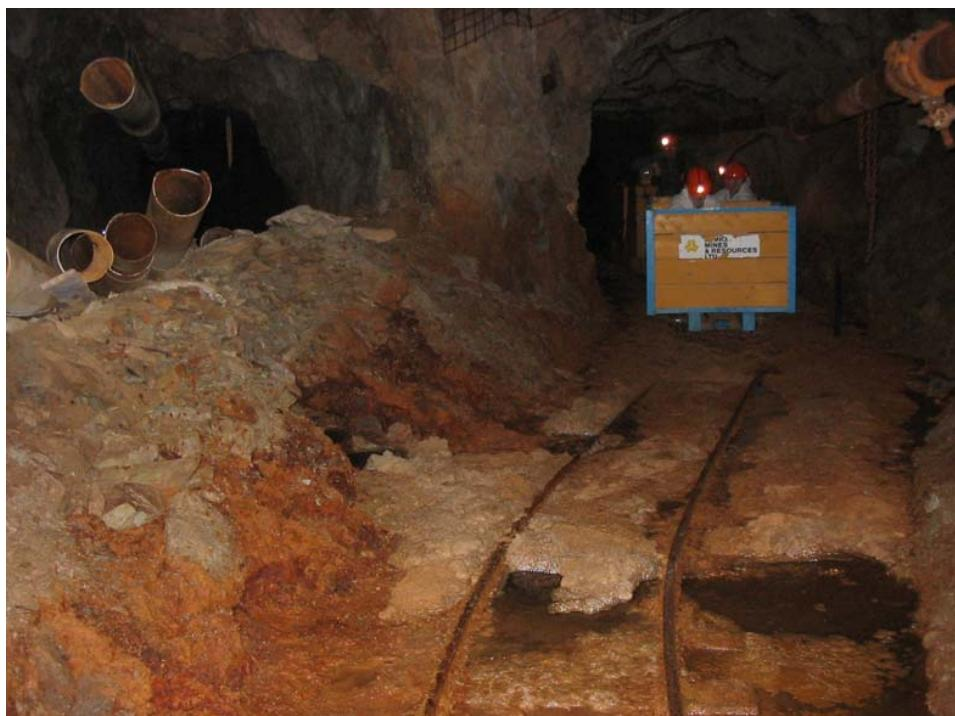
Upwelling point (under rock berm on left) where Crown shaft water reaches 800-Level
