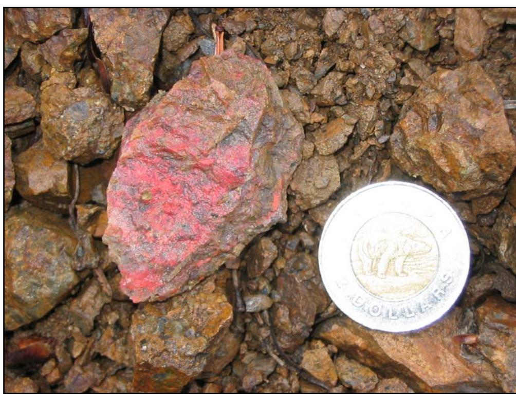
**Fig. 11.** (a) Overview of open pit at the Silverquick mercury mine showing the entrance to one of the mine adits near the right-hand side of the photo (beneath the fallen tree). (b) Cinnabar [HgS] ore and conglomerate host rock at the Silverquick Mine.
