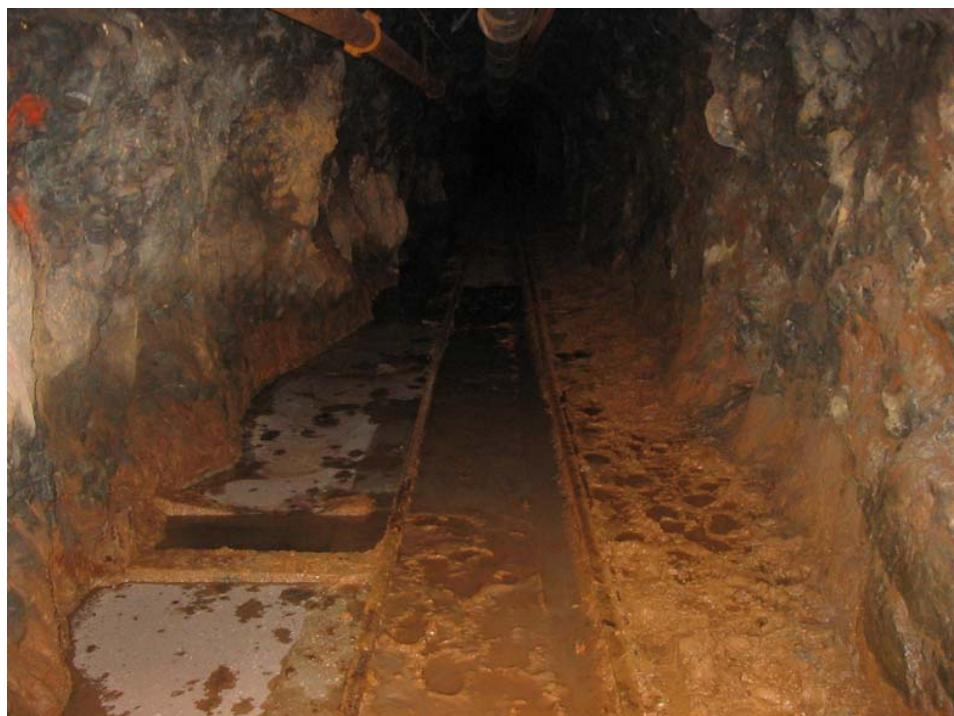
**Fe-rich sediments with slowly flowing drainage from Crown shaft on left**
