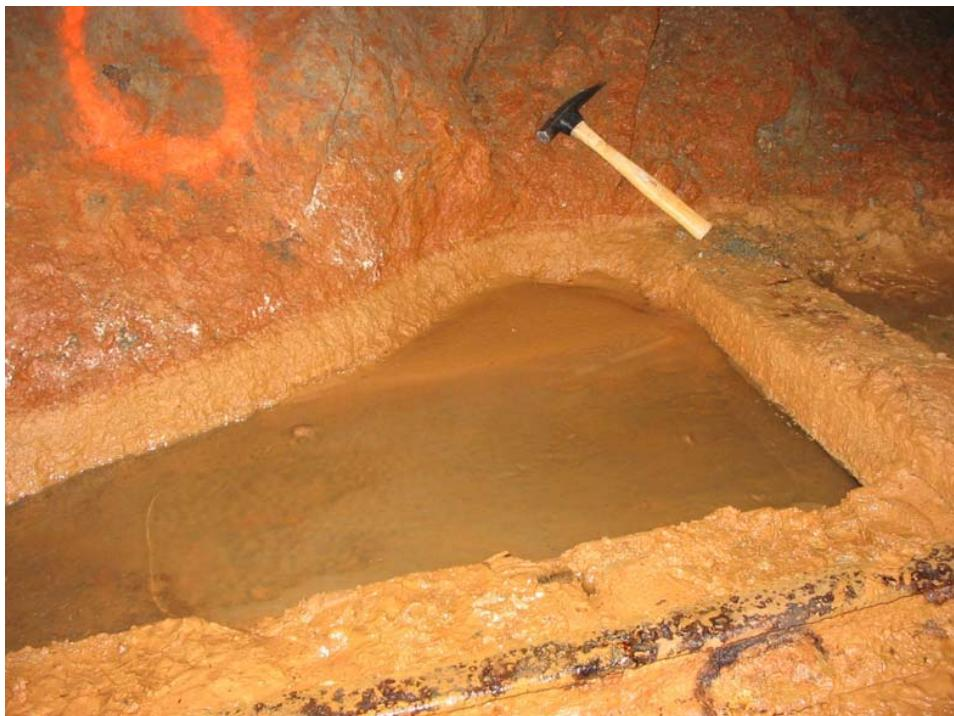
**800-Level; Fe-rich sediments adjacent to track in drainage channel**
