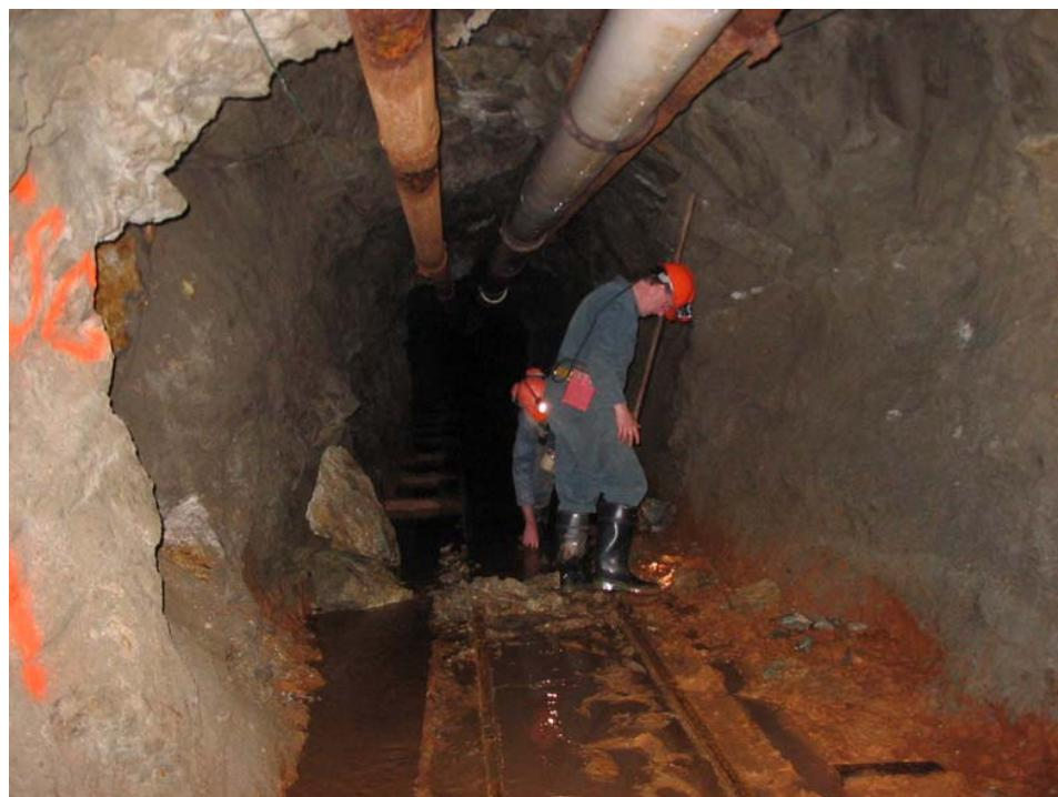
**800-Level; clearing rock fall from sediment-covered tracks**
