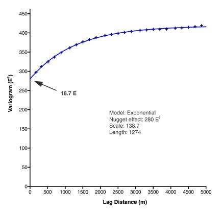
**Figure 8.** Variogram of the 75 m low-pass filtered vertical gravity-gradient data. Lag distance is the distance between each pair of data values. Crosses are calculated and the blue line is the fitted exponential model. Model parameters are given in the figure.
