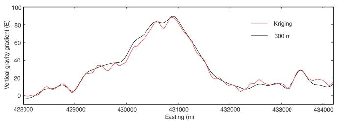
**Figure 10.** Comparison between the 300 m low-pass filtered vertical gradient of the gravity field and the vertical gradient of gravity calculated by kriging along line 11220.
