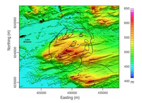
Figure 5. Digital elevation model from LIDAR and SRTM data. Black lines are major geological contacts. Crosses indicate outcrops and black areas are large outcrops. Geology adapted from Bélanger (1984) and Miller (1990).
