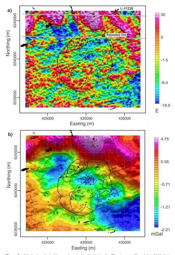
**Figure 9.** a) Vertical gradient of the gravity calculated by kriging the 75 m low-pass filtered data. b) Vertical component of the gravity field calculated by vertically integration the vertical gradient of the gravity calculated by kriging the 75 m low-pass filtered data. Grid cell is 25 m. Black lines are major geological contacts. Crosses indicate outcrop and black areas are large outcrops. Geology adapted from Bélanger (1984) and Miller (1990).
