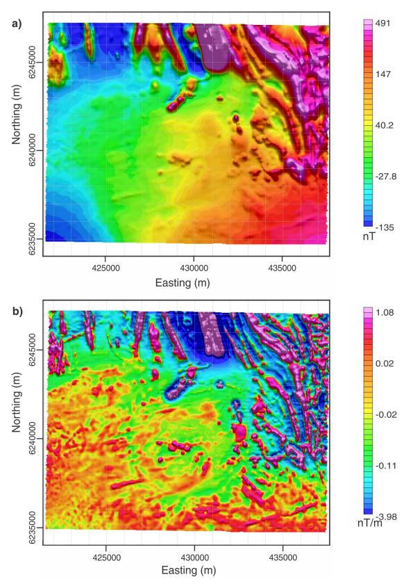
Figure 4. a) Residual total magnetic field in the Strange Lake area. b) First vertical derivative of the magnetic field in the Strange Lake area.
