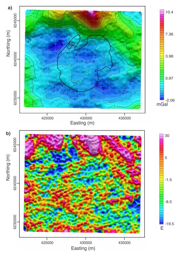
**Figure 3. a)** Vertical component of the gravity field in the Strange Lake area. The black line outlines the Strange Lake intrusive complex. M denotes mineralized zone. **b)** Vertical gradient of the gravity field in the Strange Lake area.
