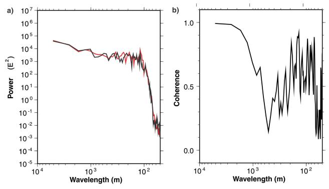
**Figure 7. a)** Spectra of  $G_{DD}$  for two of the repeat flights. Their location is shown in Figure 9a. **b)** Coherence between  $G_{DD}$  from the same two lines.
