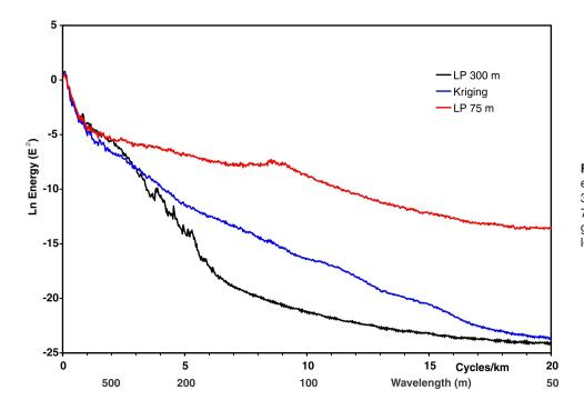
**Figure 11.** Radially averaged energy spectra of grids from the 300 m low-pass filtered data, the 75 m low-pass filtered data and grid calculated by kriging the 75 m low-pass filtered data.
