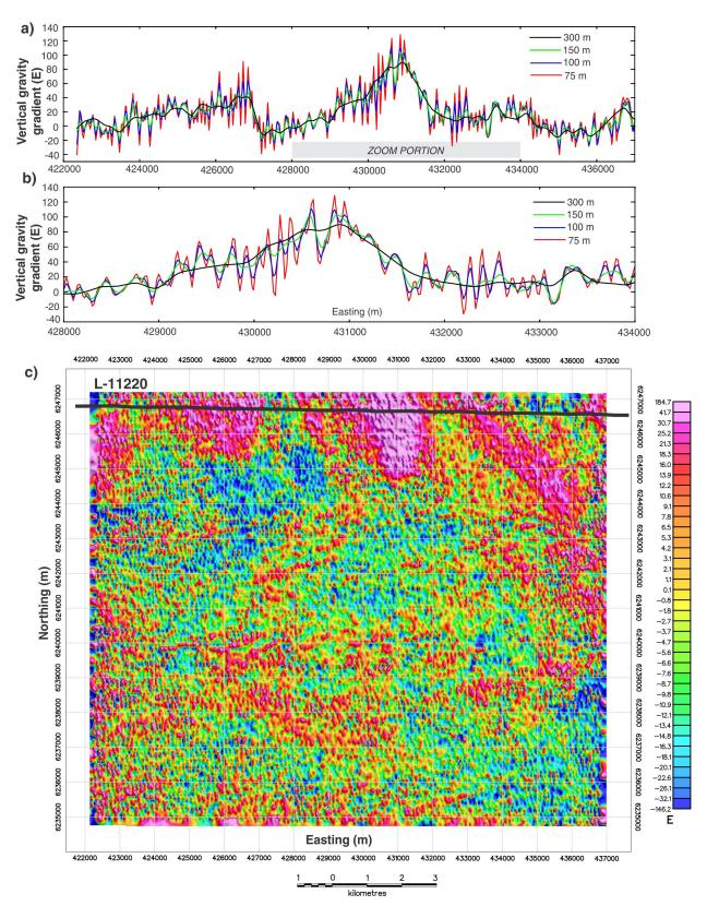
**Figure 6. a)** Vertical gravity gradient from line 11220 for different cut-off wavelengths. **b)** Detail of portion of line 11220. **c)** Vertical gravity gradient map from the 75 m low-pass filtered data. Grid cell is 25 m. The black line indicates the location of line 11220.
