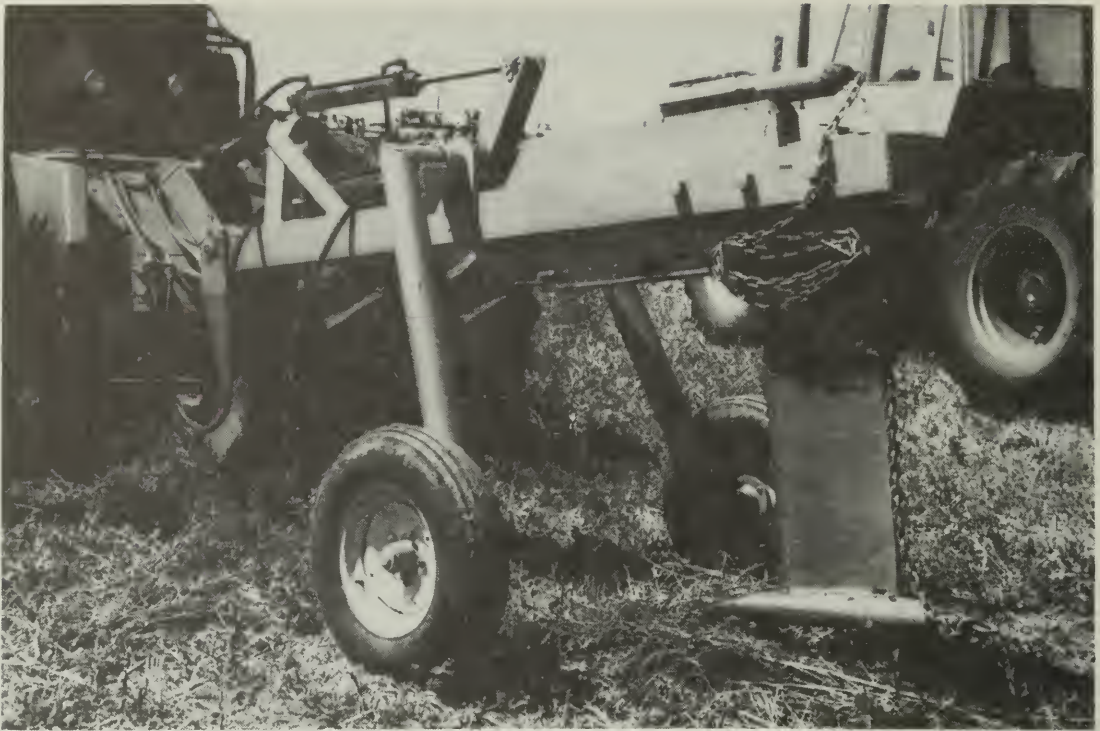
Fig. 13. Plow used for forming mole drains.
