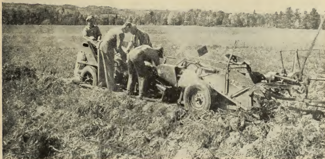
Fig. 8—Single-row power-take-off digger with bagger attachment
