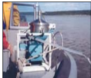
Large Volume Extraction – river water passes through centrifuge at a rate of 6.0L/min.
