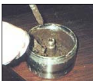
The suspended sediment is collected in the centrifuge bowl and transferred into sampling jars.
