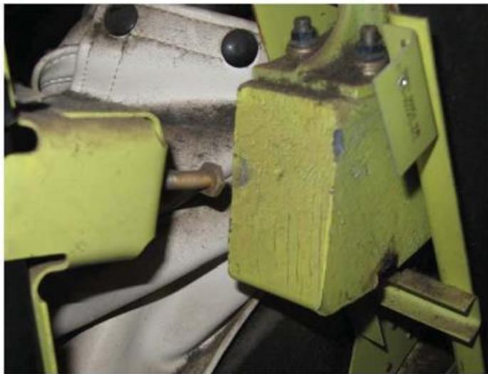
Figure 2 Partial Contact Noted on Weight, Forward of Stop Bolt
