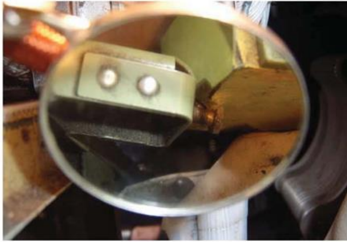
Figure 1 Stop Bolt Caught on Weight
