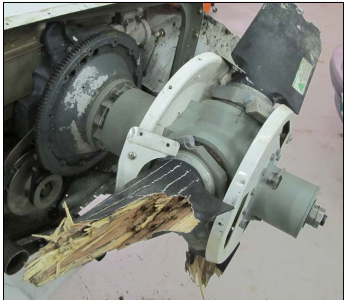
Photo 1. Propeller hub after occurrence; propeller in governing range.
