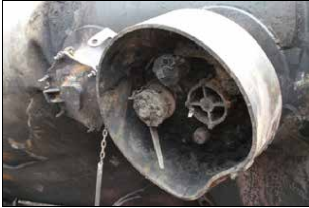
Photo 21. Protective housing providing top discontinuity protection for tank car fittings (removed cover)
