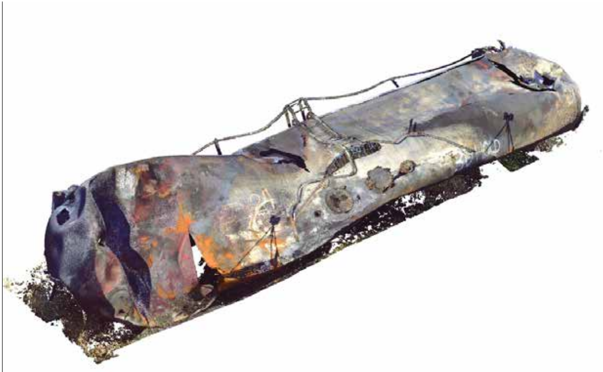
Photo 16. 3D laser scan of badly deformed tank
