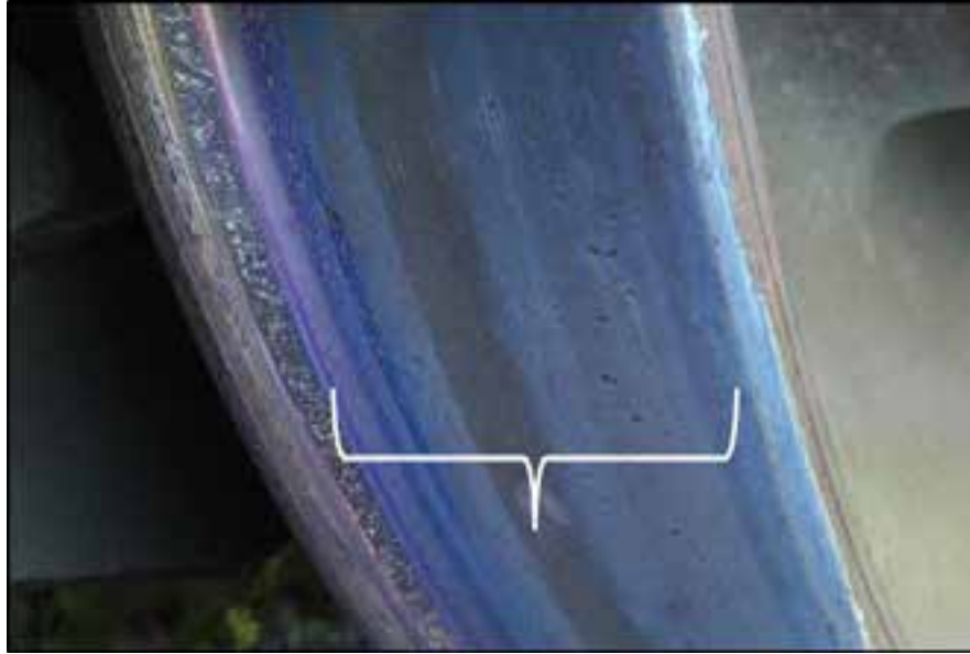
Photo 12. Blueing of locomotive wheel due to heat
