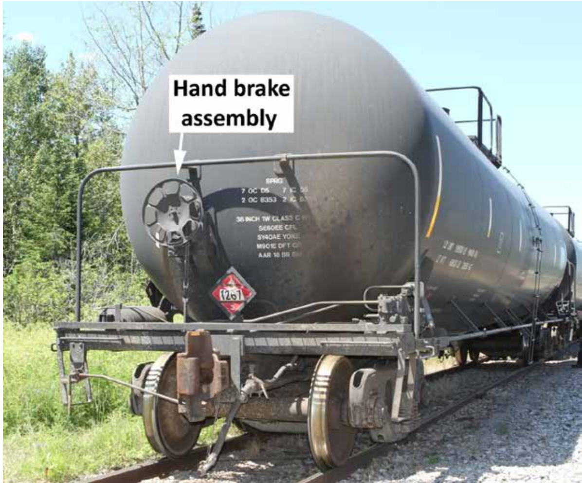
Photo 9. Hand brake assembly and wheel at the B-end of a tank car
