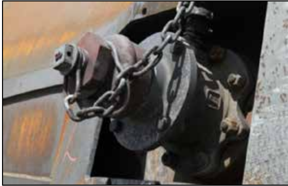
Photo 25. Bottom outlet valve
