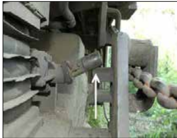
Photo 11. As the hand brake is tightened, the upward movement is intended to activate the release mechanism on the QRB valve.
