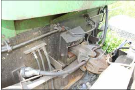
Photo 7. Pinched connector cable between couplers of second and third locomotives (occurring after the accident)
