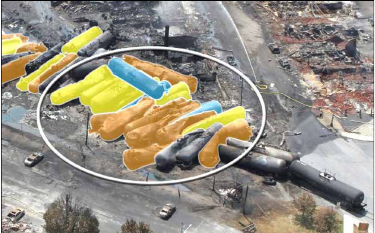
Photo 30. Concentration of large (orange) and medium (yellow) breaches toward the end of the derailment
