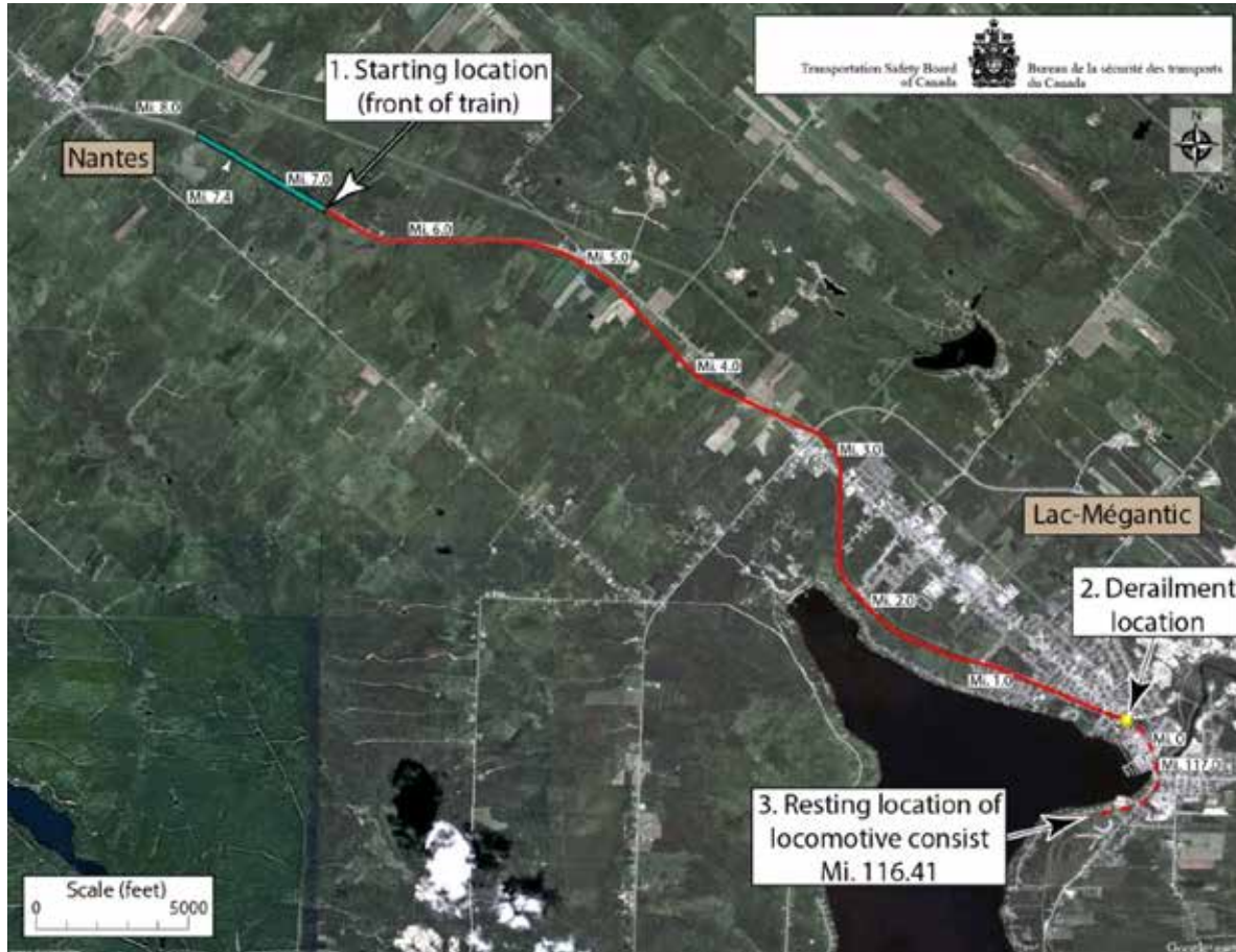
Figure 3. The 3 locations that were the focal points of the investigation: Nantes, downtown Lac-Mégantic, and the location where the locomotives came to a stop (Mile 116.41 of the Moosehead Subdivision) (source: Google Earth, with TSB annotations).
