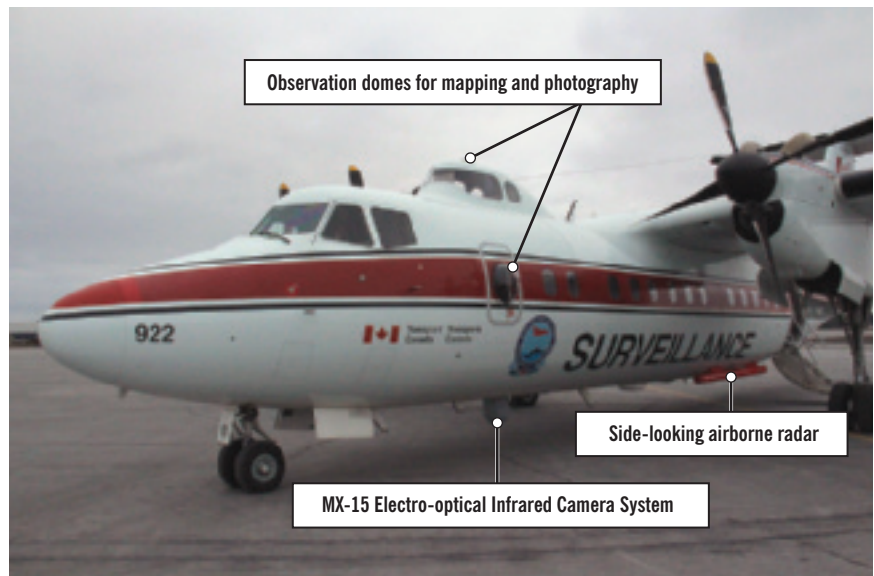
Exhibit 3.7 The National Aerial Surveillance Program's Dash 7 plane is equipped for multipurpose missions
