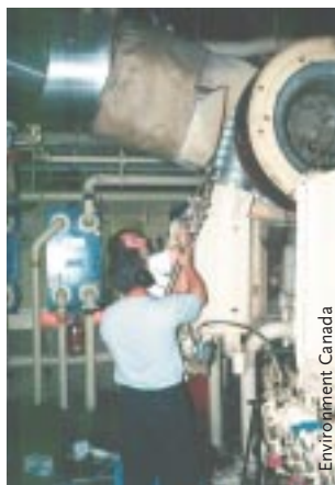
Evaluating a ferry water injection system
