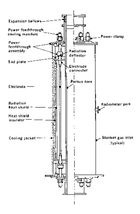
FIGURE 10 VERTICAL CROSS-SECTION OF A TYPICAL FLUID-WALL REACTOR (Thagard Research Corp., 1981)
