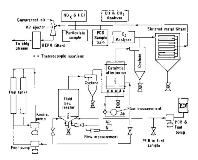
FIGURE 9 PILOT SCALE FECIDIZED BED UNIT (Rockwell Intrnational)
