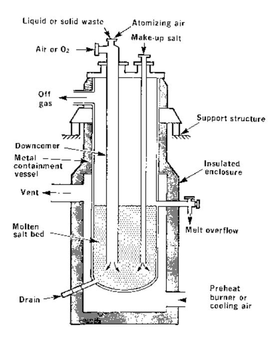
FIGURE 6 SCHEMATIC OF MOUTEN SAUT COMBUSTOR - COMMERCIAL (Rockwell International)
