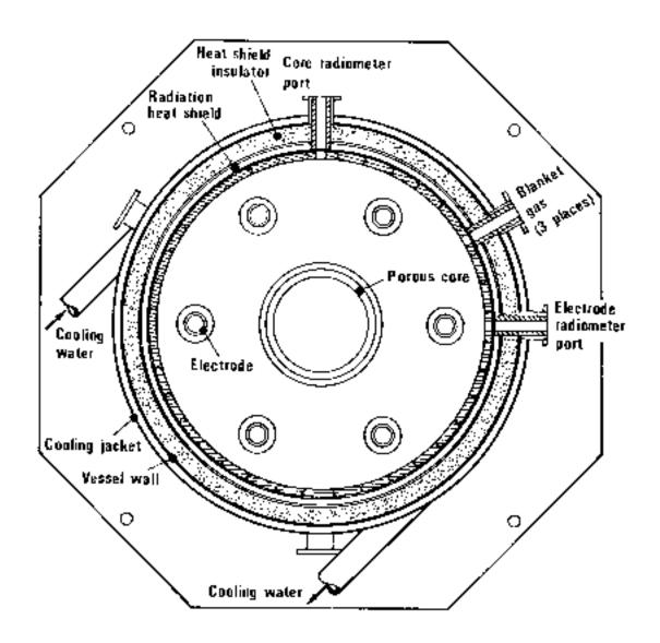
FIGURE II HORIZONTAL CROSS-SECTION OF A TYPICAL FLUID-WALL REACTOR (Thagard Research Corp., 1981)
