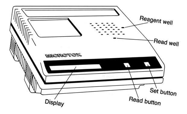
Figure 4 General Appearance of the Model 500 *Analyzer* for the Microtox Test
