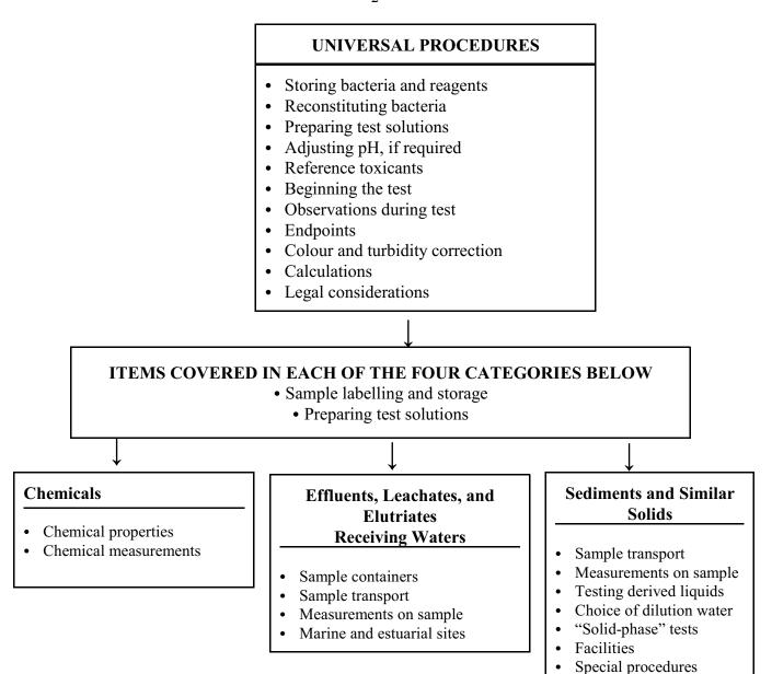
Figure 1 Diagram of Approach Taken in Delineating Test Conditions and Procedures Appropriate to Various Types of Substances
