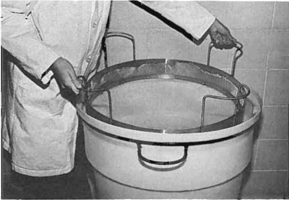
Fig. 4. Stainless steel secondary screen - for removing any larger particles of extraneous material remaining after washing roe.
