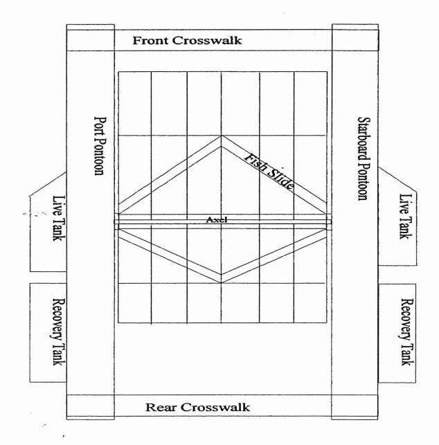
Fig. 3. Schematic diagram of fishwheel (aerial view).
