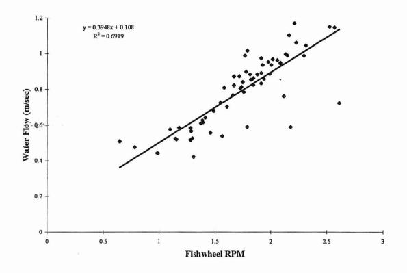
Fig. 6. Fishwheel rotational speed related to water flow, Klinaklini R., 1997.
