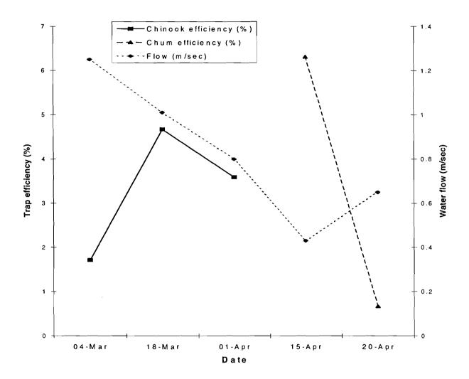
Fig. 4. Rotary trap efficiency vs water flow, pumphouse site, Cowichan River.
