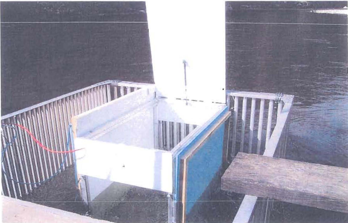
Photo Plate 2. Picture of video chamber used for enumerating returning salmon species.
