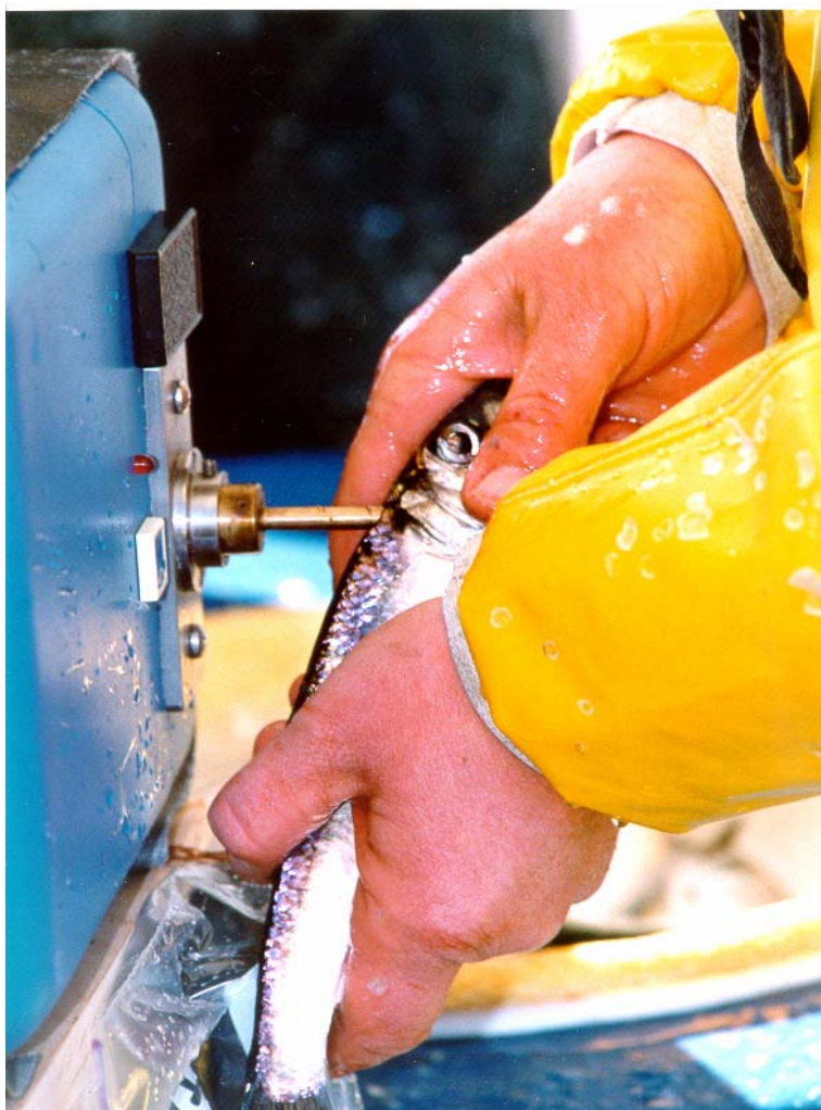
Figure 1. Photograph showing coded wire tag insertion into the nape site of a Pacific herring using a cylindrical brass needle support fixed to a Northwest Marine Technology TM Mark IV Automatic Tag Injector.
