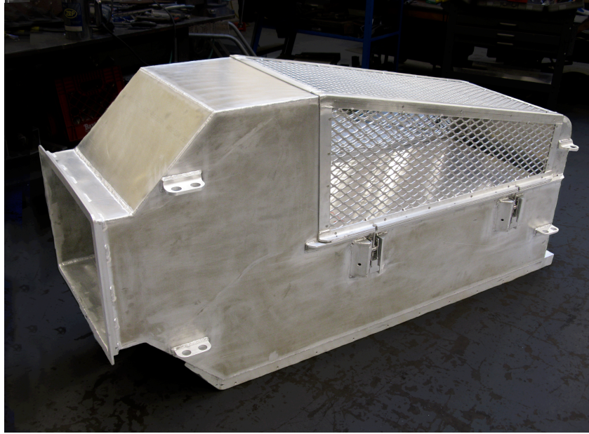
Figure II-1 : General view of “aquarium” codend during construction, with cover in place. Note slot (seen through mesh of cover, beyond rear end of deck) through which the catch drops into the tank. The shape of the ramp, leading from the entry to the deck, can be traced by the welding mark. When this photograph was taken, the vent holes had yet to be drilled.
