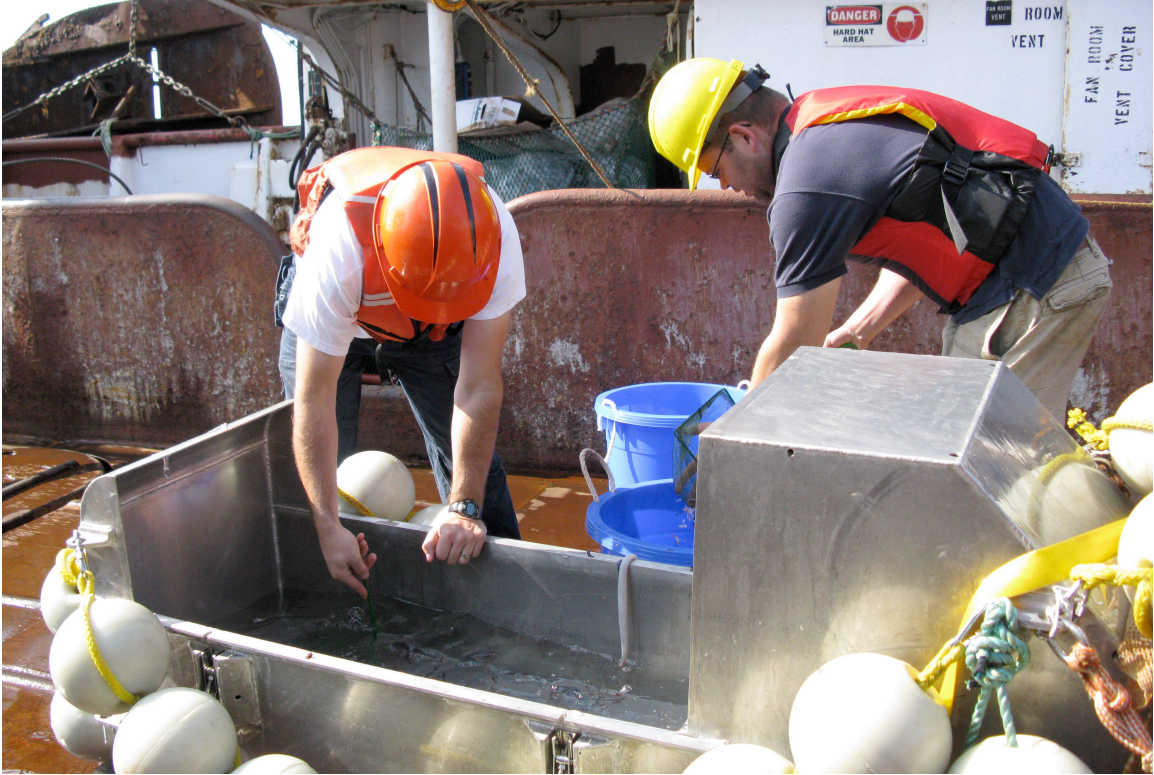
Figure II-5 : Recovering catch from the “aquarium” codend after removal of its cover
