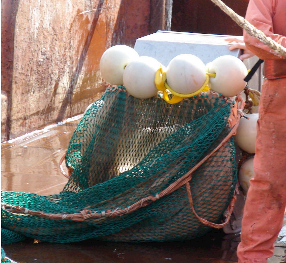
Figure II-3 : “Aquarium” codend attached to net, ready for deployment
