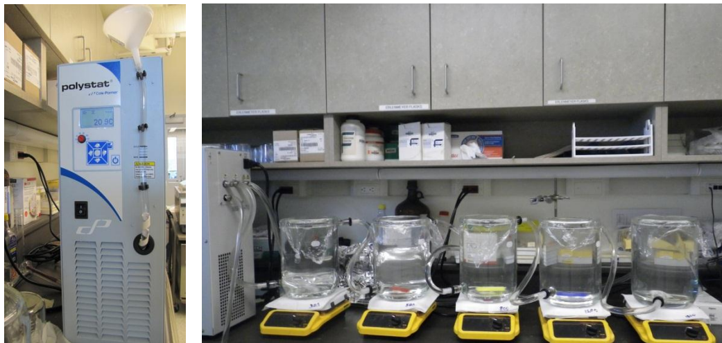
Figure 1. Polystat chiller unit and experimental setup of jacketed beakers connected to chiller unit for hydrogen peroxide degradation study.
