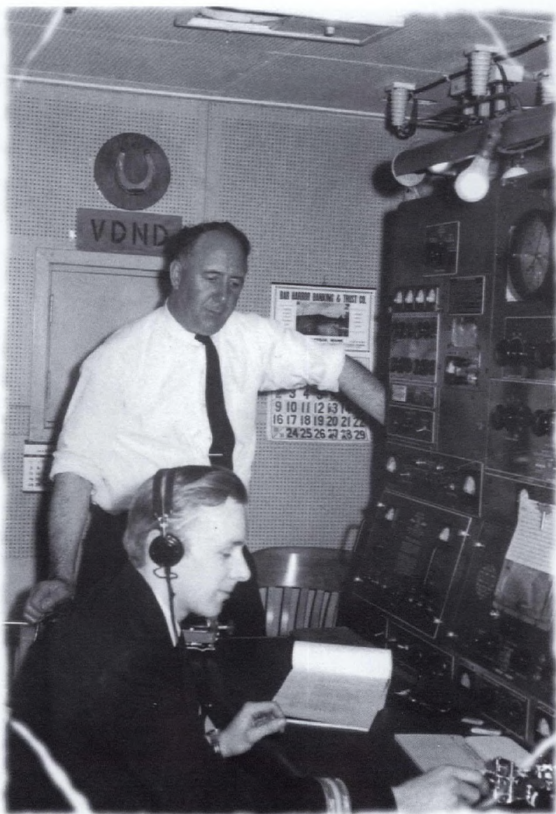
Blue Nose II radio room with radio officers Henry Whitehead (standing) and David Wail. The RCA 5U station was manufactured in the 1950s and installed on the RCMP Wood , the Bounty and the D'Iberville . The RCA unit had a 150-watt output, c. 1965. (David Wail)
