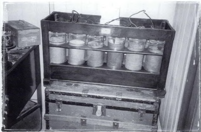
Leyden jars, type of capacitor used with the spark transmitter, 1996. (Courtesy of the S.P.A.R.C. Museum)
