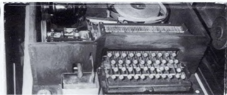
An early teletypewriter which transmitted and received written messages and data via radio relay systems. Originally developed by Frederick G. Creed, a British inventor, in the late 1890s. More often called a teletype, this instrument was used to great effect in Canada's marine radio network. (MCTS collection)
