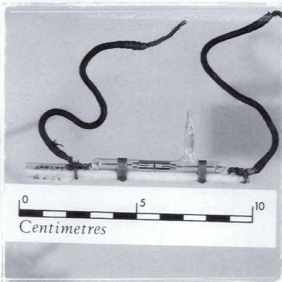
The coherer from the original receiver on the cableship Mackay-Bennett , assigned to study the useful range of the Camperdown station. Marconi installed the transmitter and receiver on the Mackay-Bennett in 1899 when the vessel was sent to New York to observe and report the famous yacht race between Sir Thomas Lipton's first Shamrock and the defending Columbia . (Courtesy of Dalhousie University Archives, Thomas Raddall Collection)
