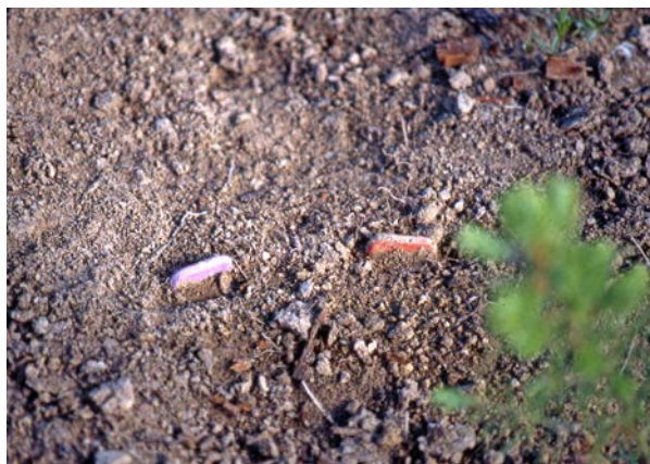
Figure 8. PRS™ probe pair installed in soil.
