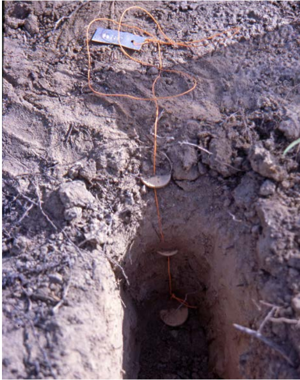
Figure 9. Installed set of three tongue depressors.
