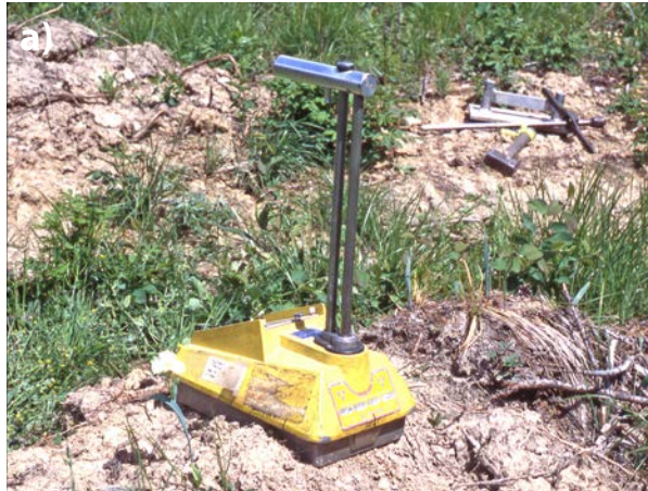
Figure 7. Measuring bulk density a) using a Troxler gauge on a deposit and b) using the sand replacement technique.
