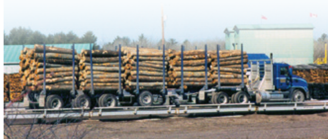
Truck loaded with logs on a weigh scale. The volume of logs is calculated from the weight of the load on the truck.
