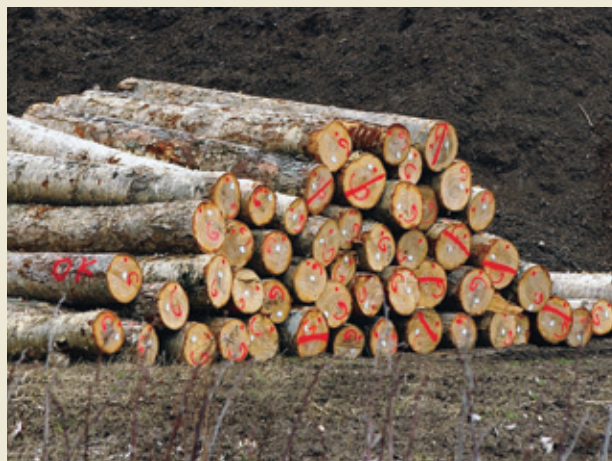
Yellow birch logs stamped and tagged to ensure tracking of valuable logs throughout the process from woods to mill to product.
