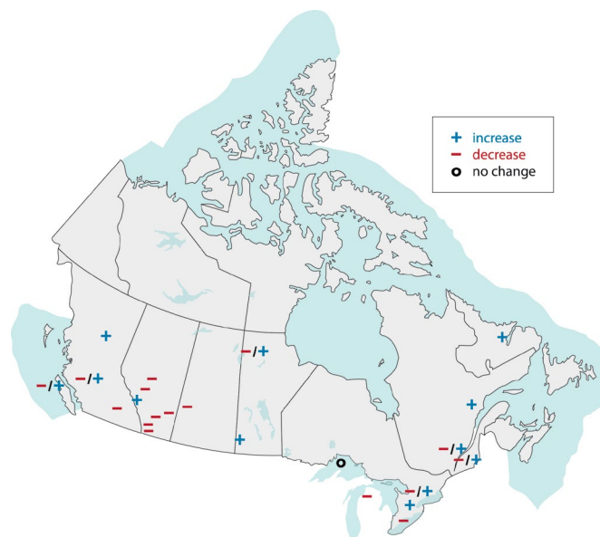
FIGURE 23: Projected changes in annual runoff for the 2050s period, from research published during 2008-2013. A '-/+' means that for a particular study location, scenario projections include both decreases and increases. See Table 2 for study references.
