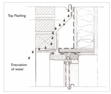
Figure I Top Flashing
