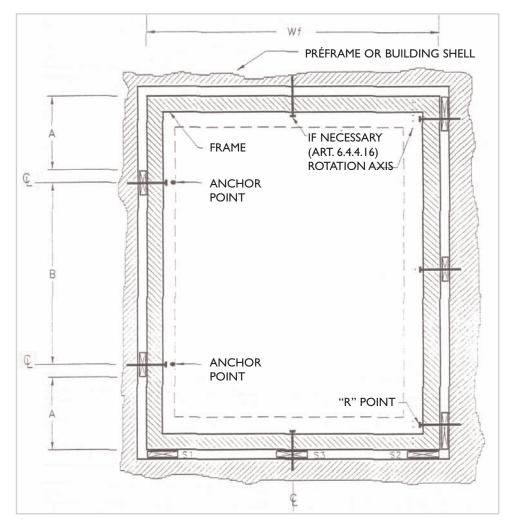
Figure 3 Shims for Casement Windows
