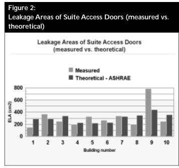
limits for fire doors, but always greater than allowable National Building Code of Canada (NBC) limits for fire doors and greater than allowable NFPA limits for smoke-control doors. Some buildings had considerable differences between theoretical and measured door leakage areas, as shown in Figure 2.
