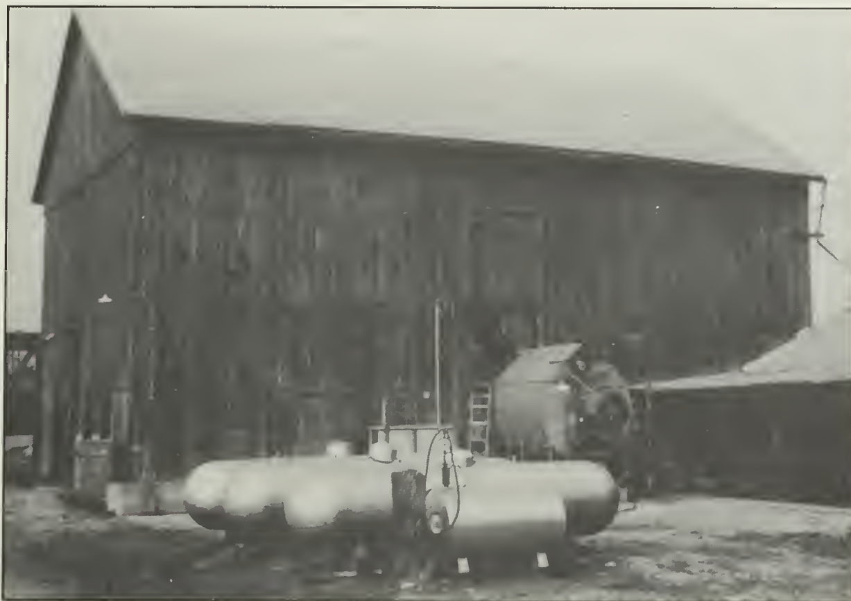
Fig. 6.25 Heated Air Grain Drying with Propane
