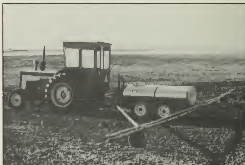
Fig. 6.20 A Farm Sprayer for Herbicide Application
