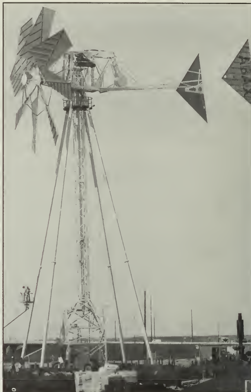
Fig. 8.4 Prototype of a Large Scale Canadian Wind Pump. (Courtesy Deltx Corporation, Calgary, Alberta).
