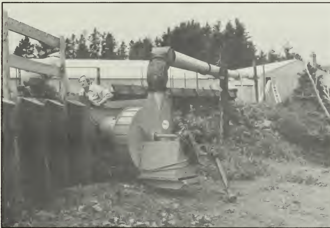
Fig. 8.10 A Wood Gasifier for Farm Heating
