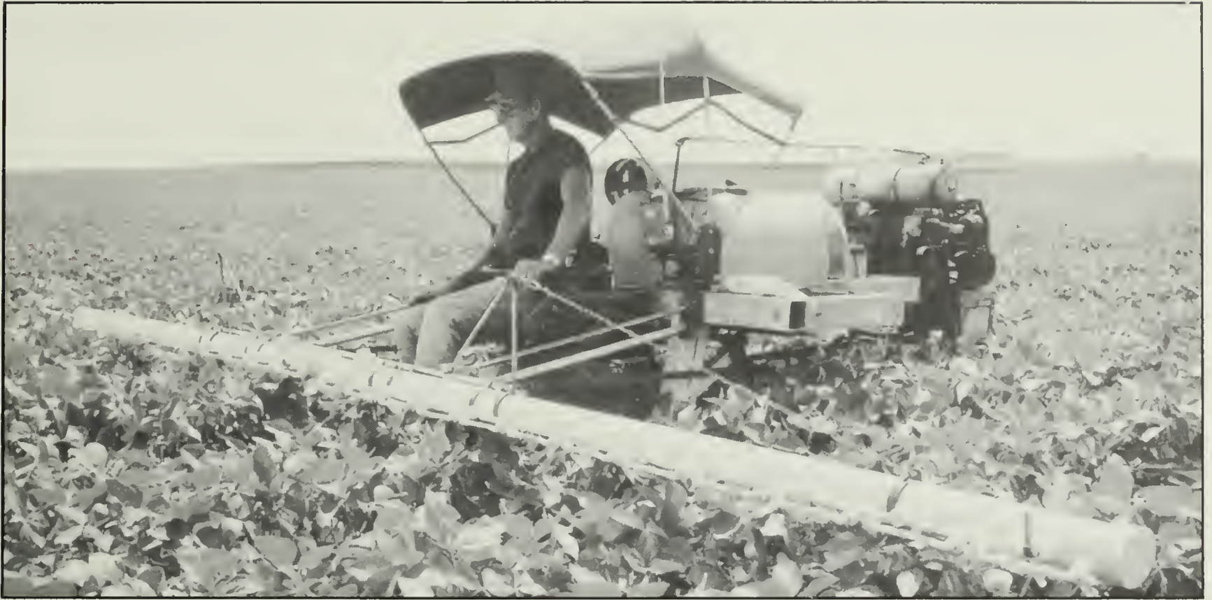
Fig. 6.22 A Rope-Wick Herbicide Applicator
