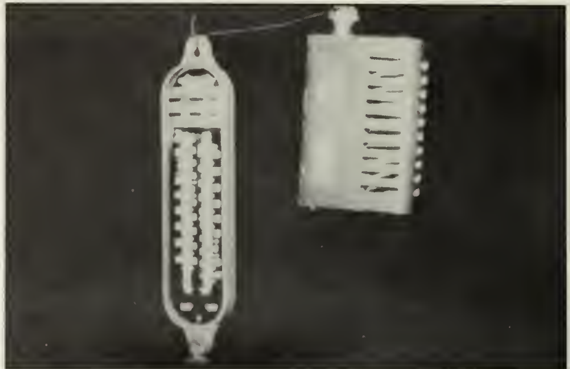
Fig. 7.12 Thermostats Should be Checked Regularly with a Good Thermometer.
