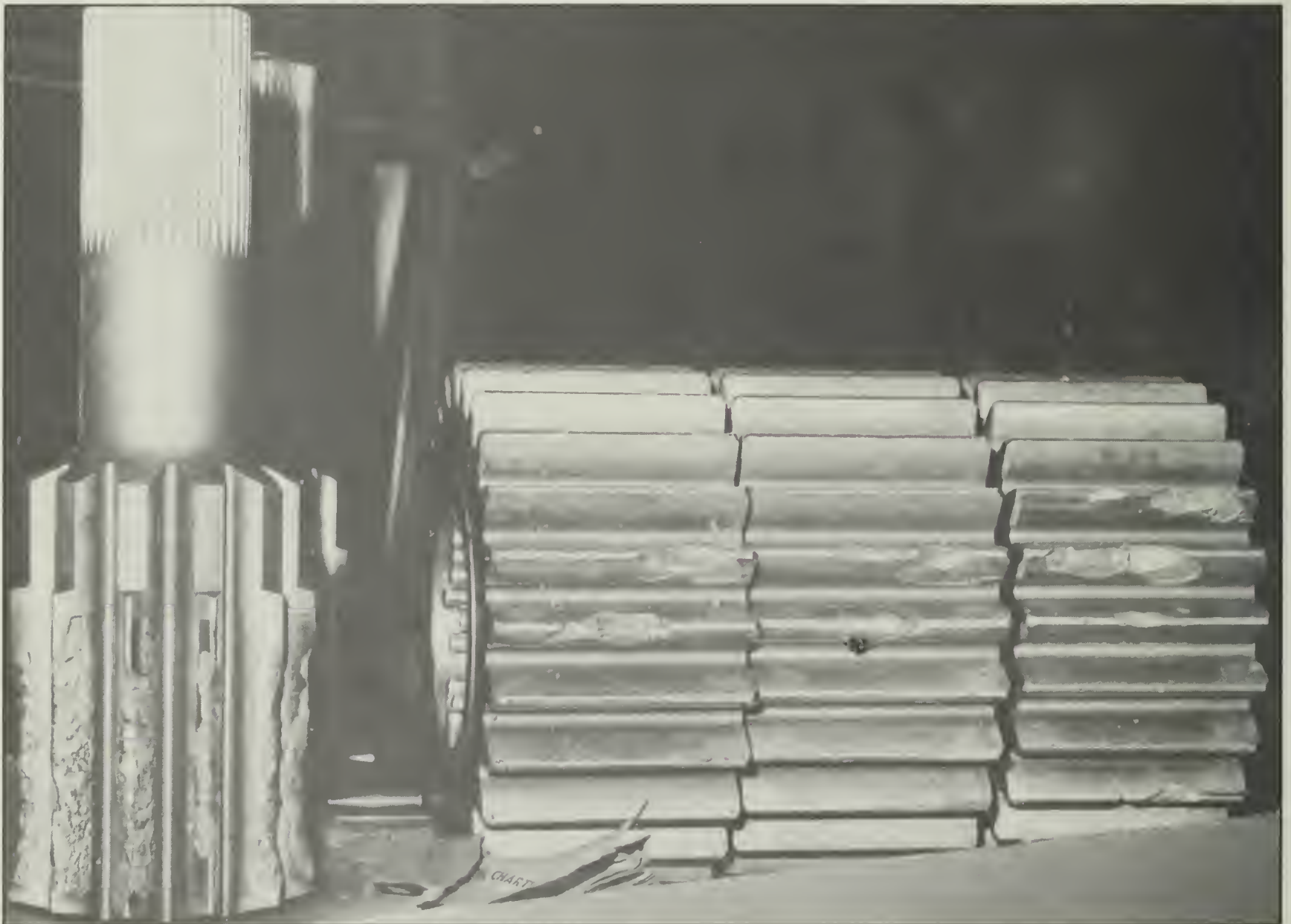
Fig. 5.12 Overballasting Causes Expensive Driveline Failures.
